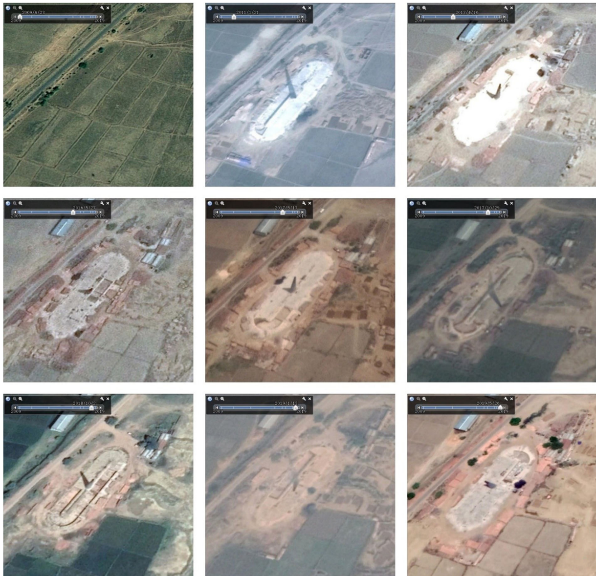
Fig. 1 The historical satellite imagery in the Google Earth Engine platform of the Bull's Trench brick kiln mapped at 24°41'15"N, 84°30'24"E (Bihar, India). Data from Google, © 2021, CNES/Airbus, Maxar Technologies. This kiln has not been built in the earliest image of this location (acquired on June 23, 2009), but had been built by the time the image dated January 21, 2011 was acquired; this kiln was inferred to be built between these two dates. The rest of the images illustrate how the same kiln appears throughout the satellite record in Google Earth, through to the latest date—26 May 2019. Note that the temporal frequency of kiln capture increases over time as the use of VHR satellite imagery becomes more common place.
