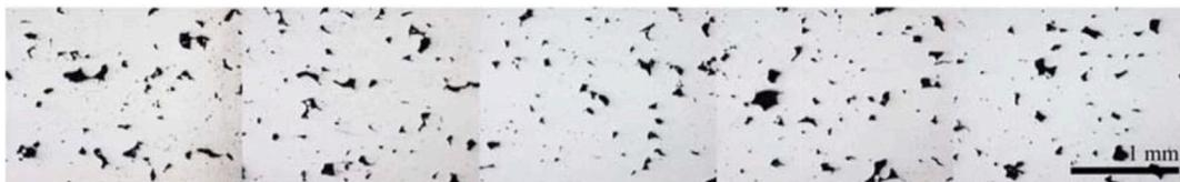
**Fig. 8.** Optical micrographs of a laser powder bed fused specimen [58]. Porosity and other defects are clearly present in the material. These can be easily detected using optical micrography. However, caution should be taken when considering softer materials as smearing can serve to obscure pores. (Process parameters used: 295 W, 2250 mm/s 0.11 mm layer height.)
