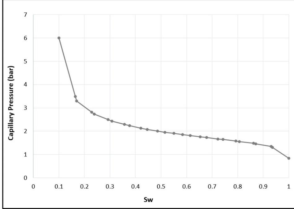
**Figure 4.** A capillary pressure curve that was used in the validated base case.
