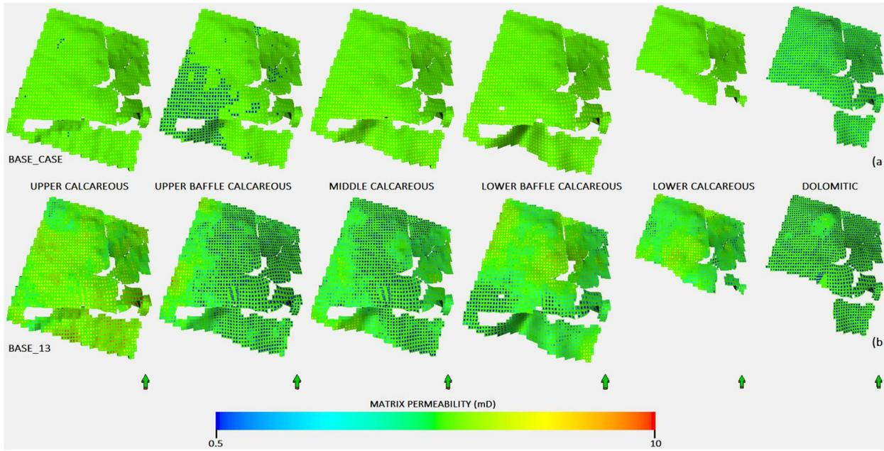
**Figure 8.** Comparison of matrix permeability distribution in X-direction for the homogeneous base case with that for the heterogeneous case (base\_13).
