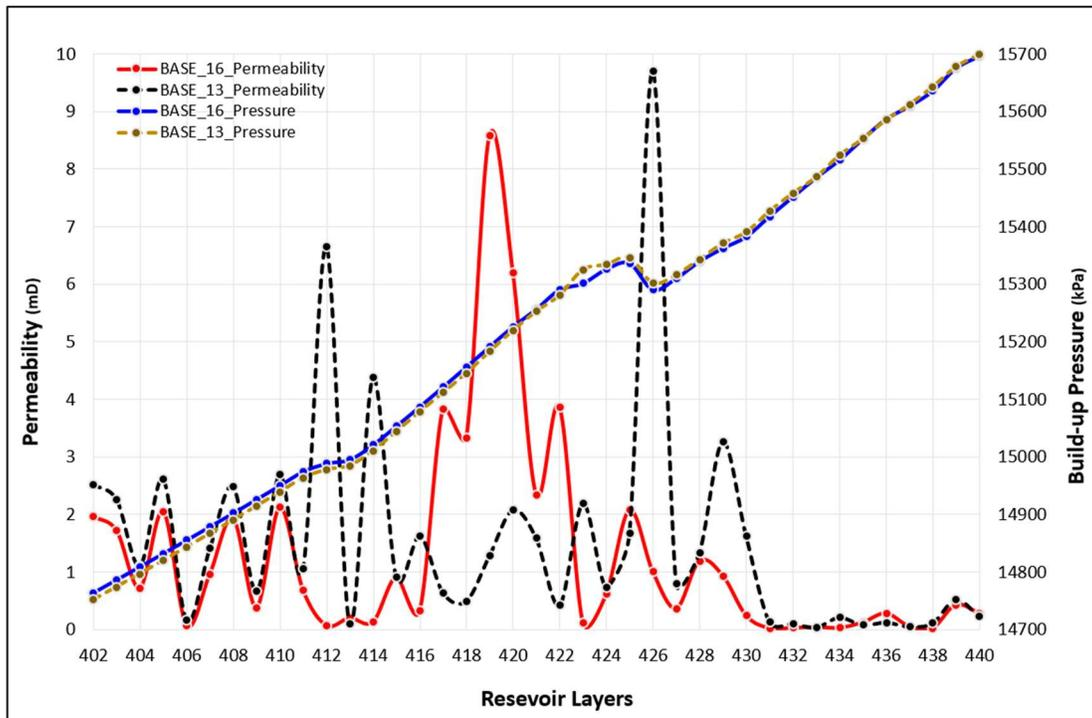
**Figure 10.** The relationship between permeability and pressure build-up for each layer of the reservoir as it was recorded in the grid cells that were penetrated by the injection well. The pressure build-up is inversely proportional to the matrix permeability in this case.
