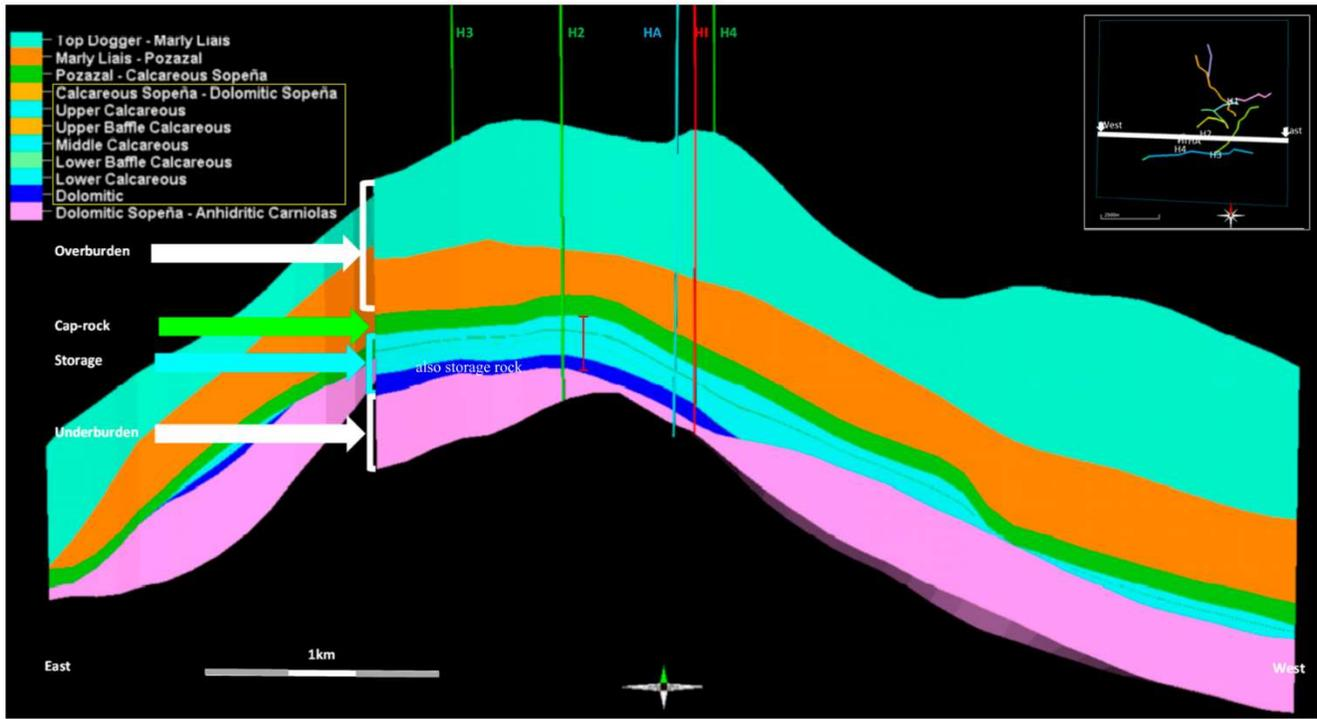
**Figure 1.** Vertical cross-section of the geological model of the Hontomín storage complex; The HA and HI newly-drilled wells are the observation & injection wells, respectively, while well H1 to H4 are legacy wells [23]. The legacy wells were used to confirm the geological sections & reservoir geometry.
