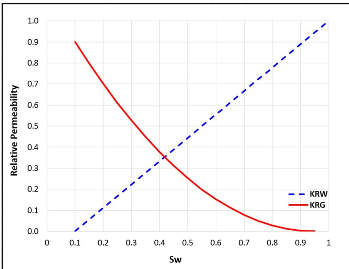
**Figure 3.** The relative permeability curves for matrix and fractures that were used in the history matching process.
