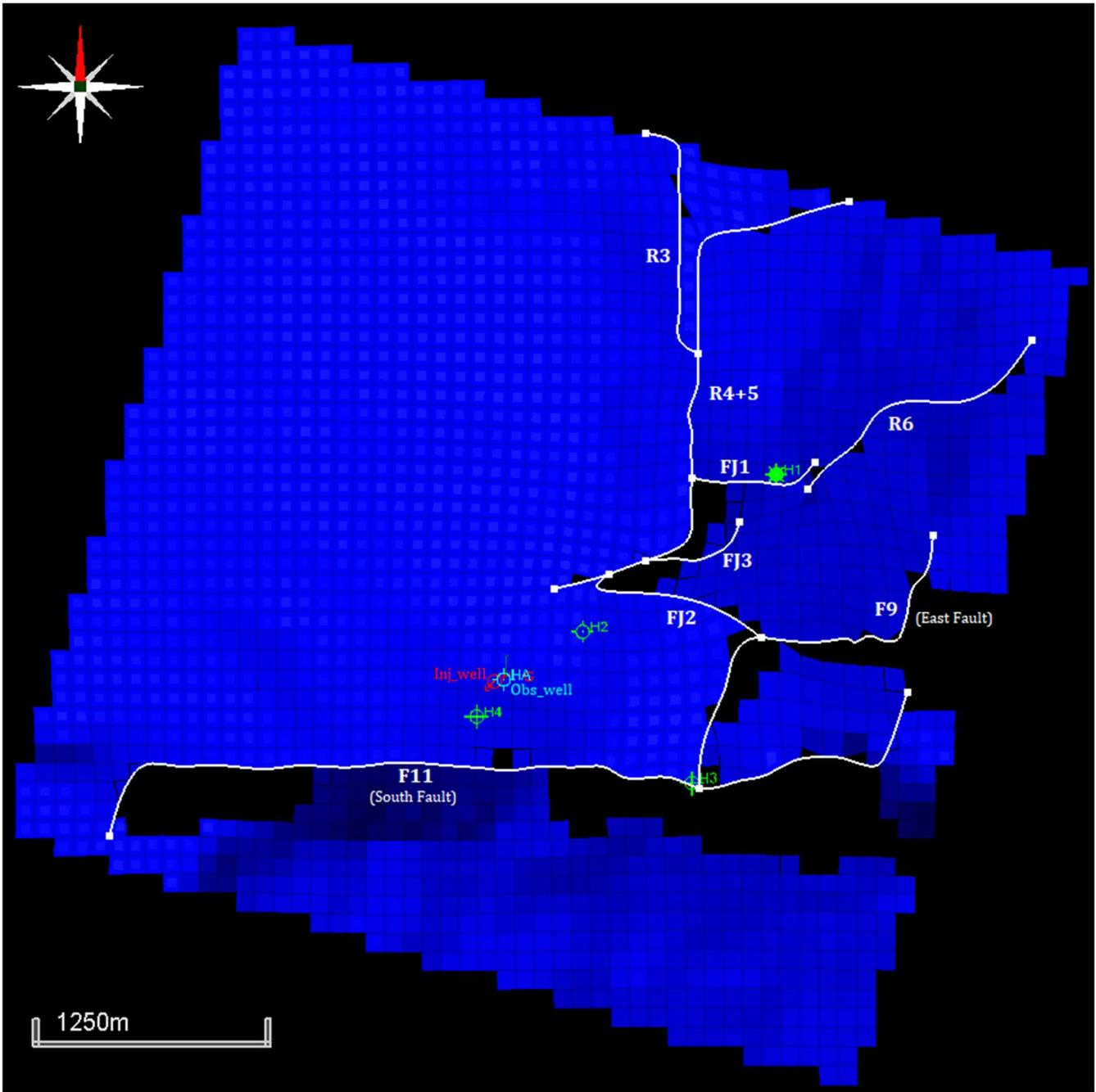
**Figure 2.** Location of wells and the extensions of all the eight faults within the Hontomín geological model in Petrel. F11 (South Fault) is located in the south, while the F9 (East Fault) is located on the east side and controls the structural extension of the reservoir in the south-east direction.
