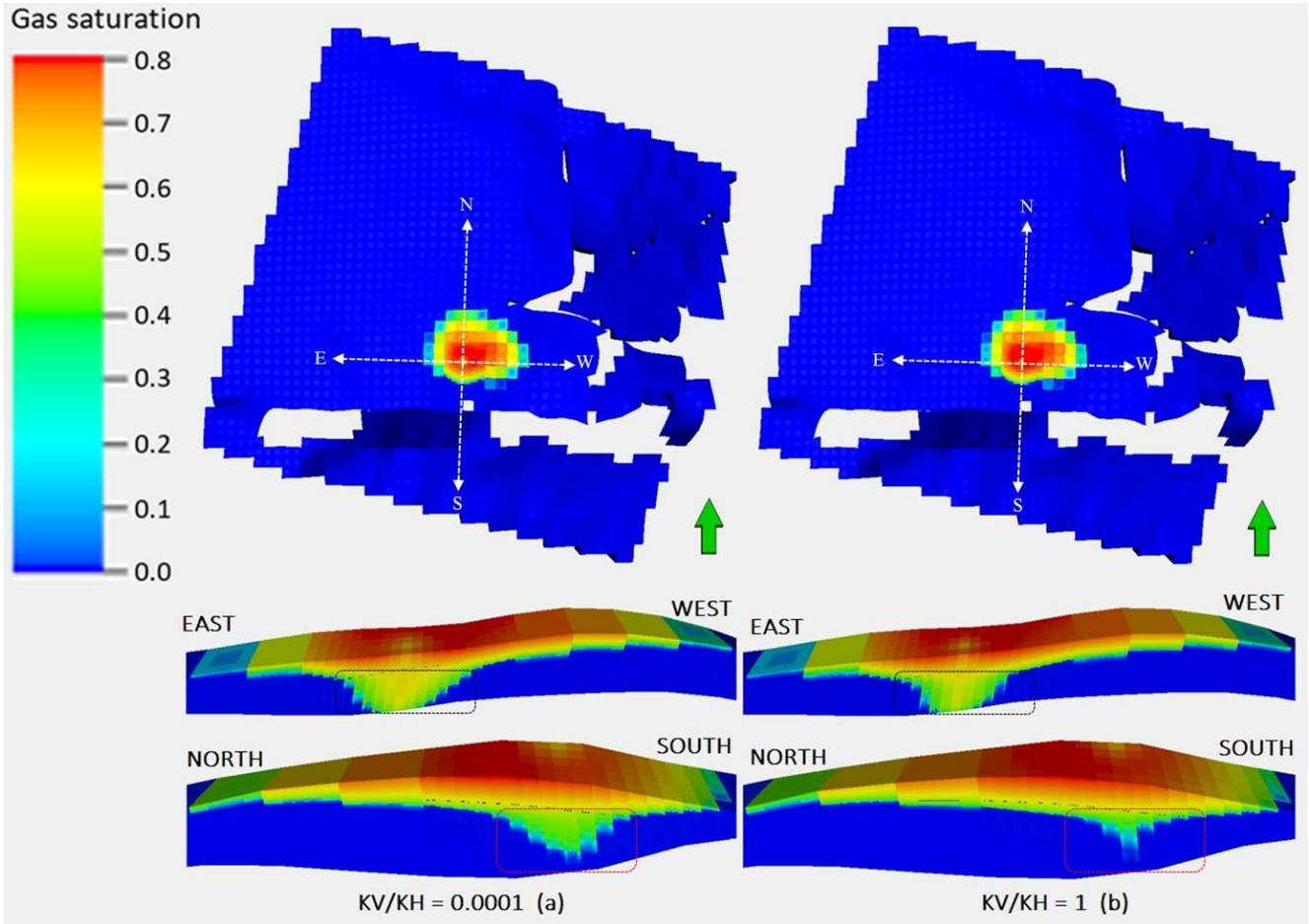
**Figure 17.** Movement of CO<sub>2</sub> plume in the horizontal and vertical direction when  $k_v/k_h$  increased from 0.0001 to 1 (a) and (b) respectively during gas injection for 50 years in the base case. The E-W & N-S segments of the reservoir are taken from the part in which the injection well is located. The black rectangles shown are to highlight the key differences between cases.
