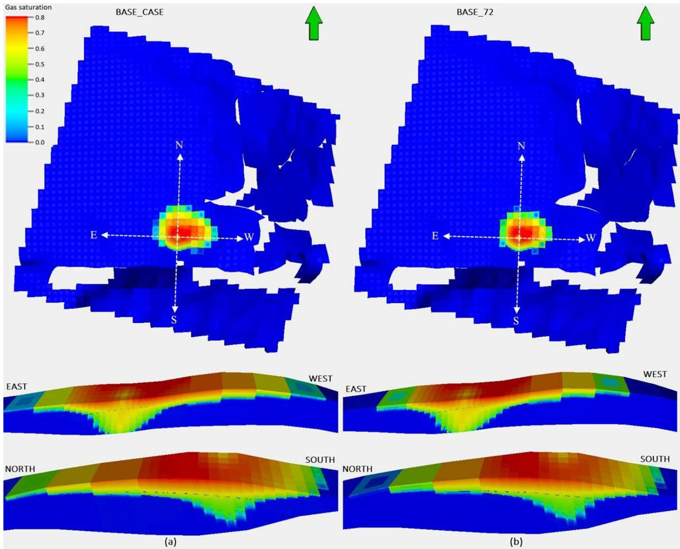
**Figure 13.** Part (a) shows the migration of CO<sub>2</sub> plume in the base case and part (b) shows migration in case base\_72 over 50 years of gas injection. The same volume of CO<sub>2</sub> was injected but the migration of plume was different in both cases as porosity changes.
