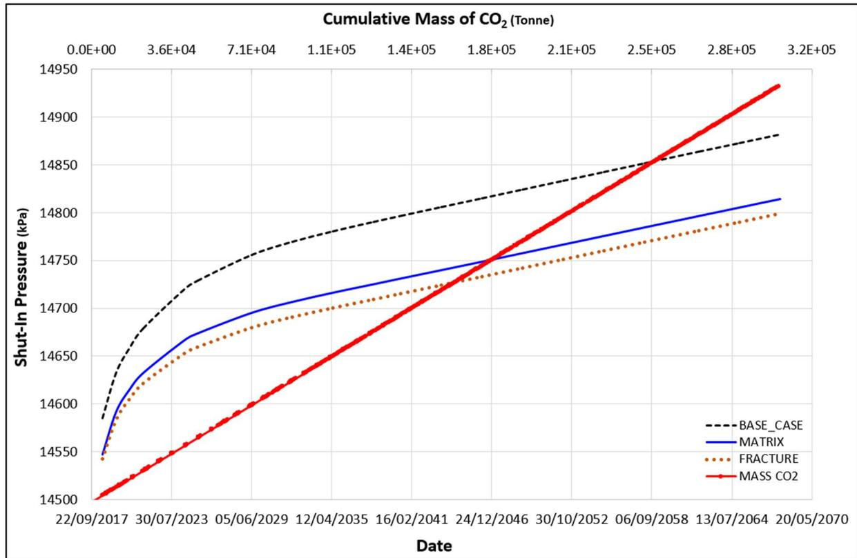
**Figure 16.** Comparison of reservoir shut-in pressures over 50 years of gas injection for the base case when increasing either matrix or fracture permeability in the Y-direction by a factor of two. The red dotted line shows the cumulative mass injection of CO<sub>2</sub> for fifty years.
