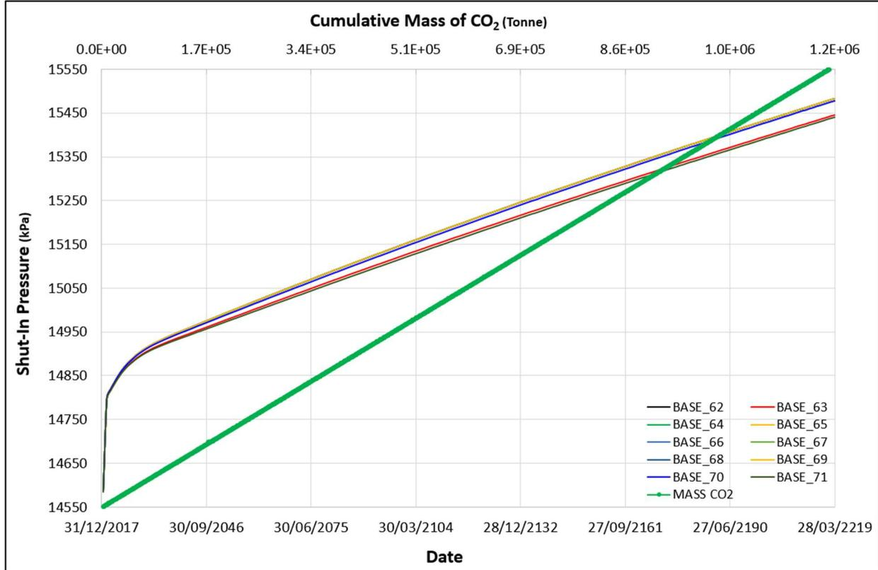
**Figure 20.** Influence of transmissibility of faults F11 and R4+5 on reservoir and injection pressure compared to the fully sealing case over 200 years of gas injection. The cases denoted base\_63 and base\_70 represent when either the fault F11 or fault R4+5, respectively, were fully transmissive as compared to base\_62 which corresponds to a fully sealing state for both faults.
