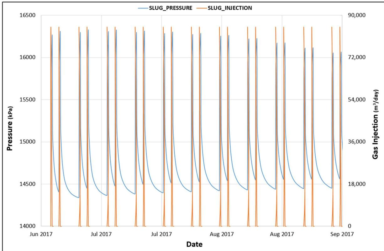
**Figure 7.** Small scale display of CO<sub>2</sub> slug injection rate and pressure during the WAG process in the homogeneous base case.
