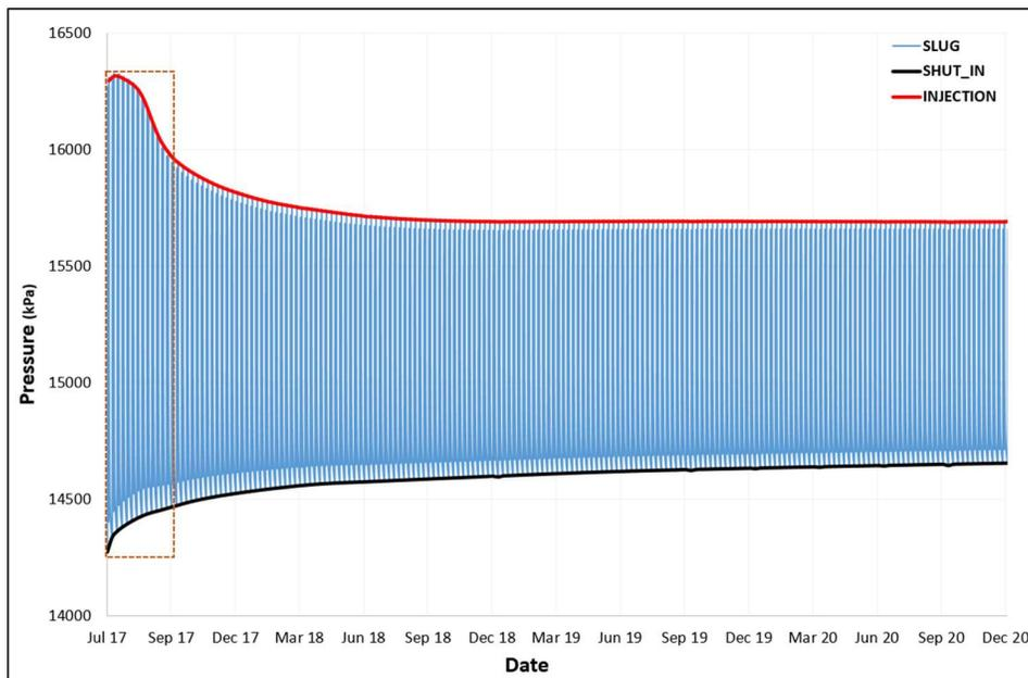
**Figure 6.** Build-up and shut-in reservoir pressures during water alternating gas slug injections in the homogeneous base case. The boxed part of the plot is shown on a smaller scale in figure 7.
