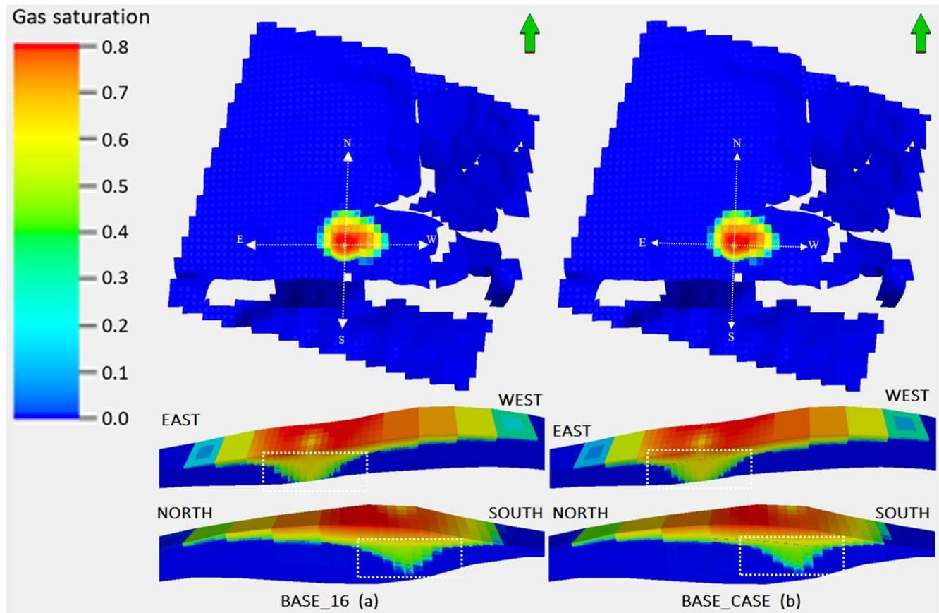
**Figure 12.** Part (a) shows the migration of CO<sub>2</sub> plume in base\_16 and part (b) shows the migration of CO<sub>2</sub> plume in the homogeneous base case over 50 years of injection. The same volume of CO<sub>2</sub> was injected in both cases but the migration of plume was different in the heterogeneous case because of the variation in matrix permeability distribution.
