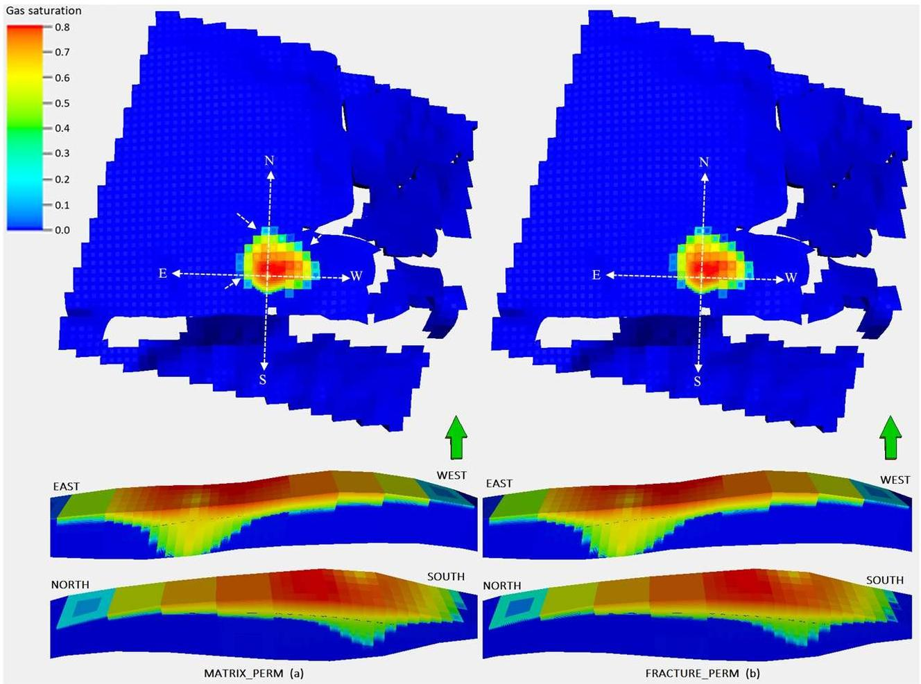
**Figure 15.** Comparison of CO<sub>2</sub> plume migration in all directions from the injection well when a change in the matrix or fracture permeability in the y-direction is twice higher compared to the base case in part (a) and (b) respectively. The CO<sub>2</sub> plume spread in both cases is almost identical but there is slightly higher gas saturation in the matrix case at the outer periphery of the plume and pointed out with the arrows.
