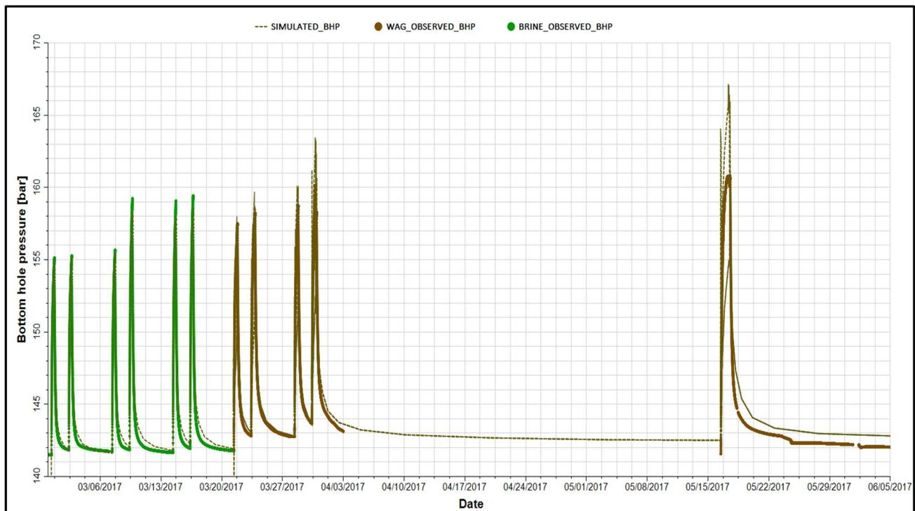
**Figure 5.** History matching of the simulated bottom-hole pressure for the Hontomín model with brine and WAG well test observed data respectively for 2017.
