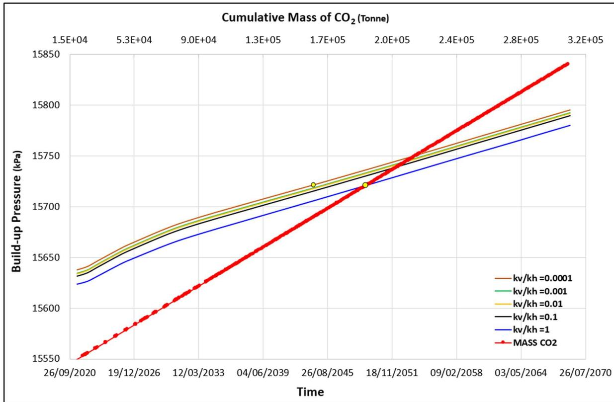
**Figure 18.** Simulated pressure build-up over 50 years of gas injection when  $k_v/k_h$  of the matrix was gradually decreased from 1 to 0.0001 for the base case. The plot shows pressure build-up and cumulative mass injection during the prediction phase.
