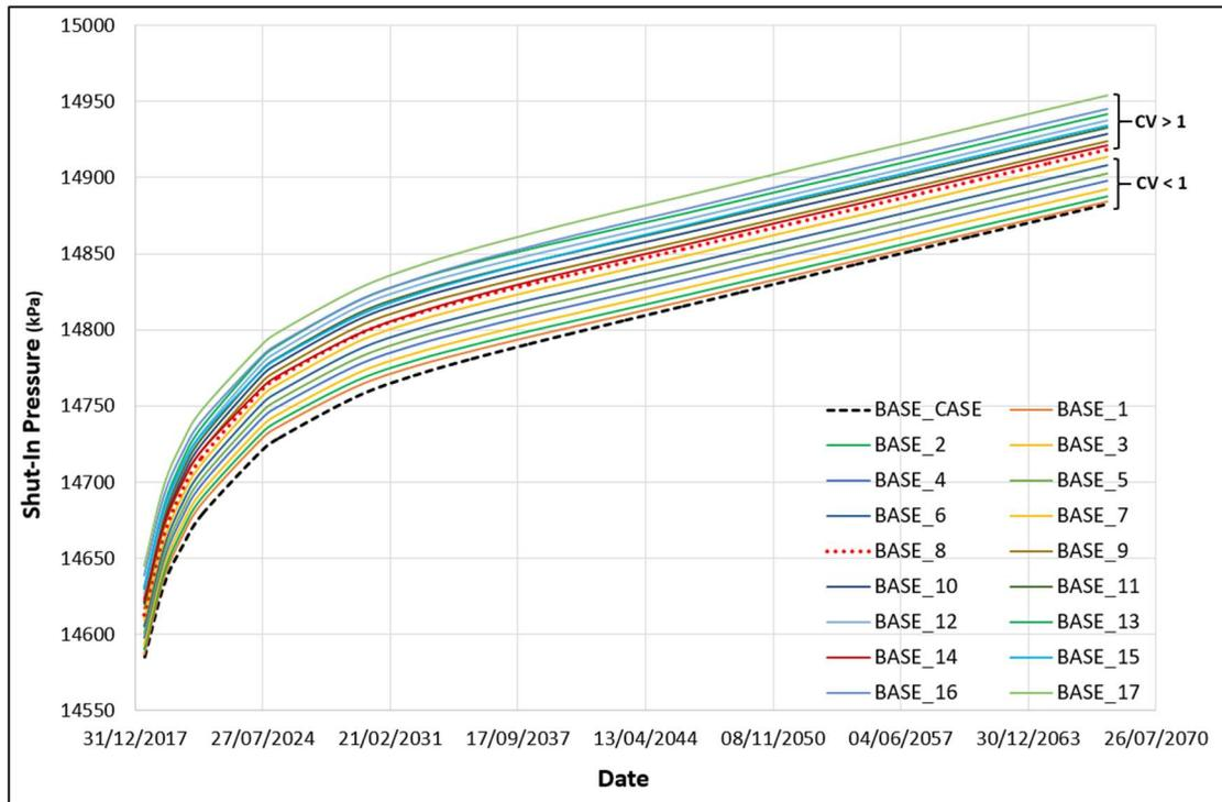
**Figure 9.** The variation of reservoir shut-in pressure, over 50 years of gas injection, with increased heterogeneity in matrix permeability in the horizontal direction.
