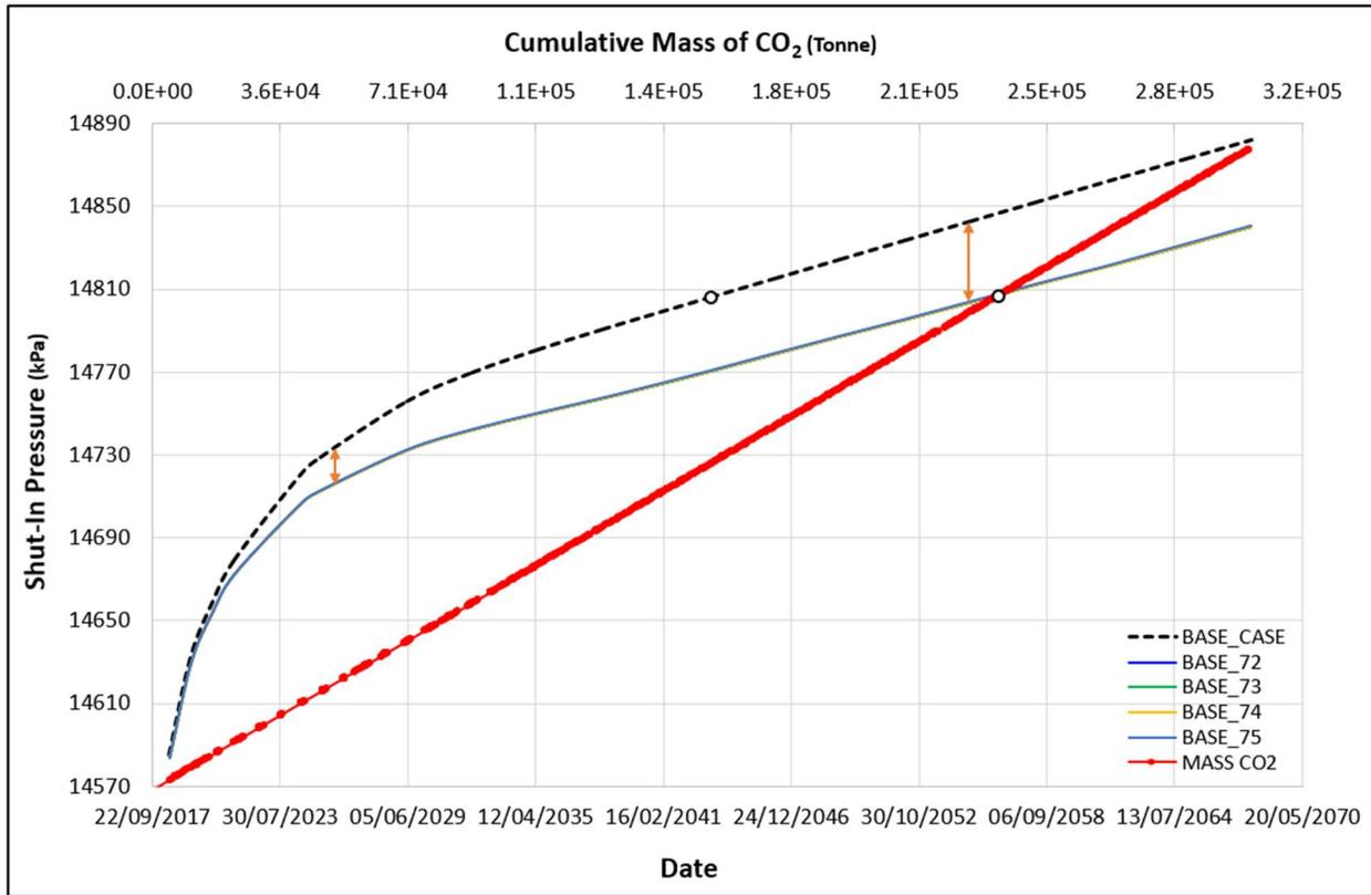
**Figure 14.** Reservoir shut-in pressure versus the cumulative injected mass of CO<sub>2</sub> for a similar time period. The heterogeneity of the simulated models based on the variation in matrix porosity.
