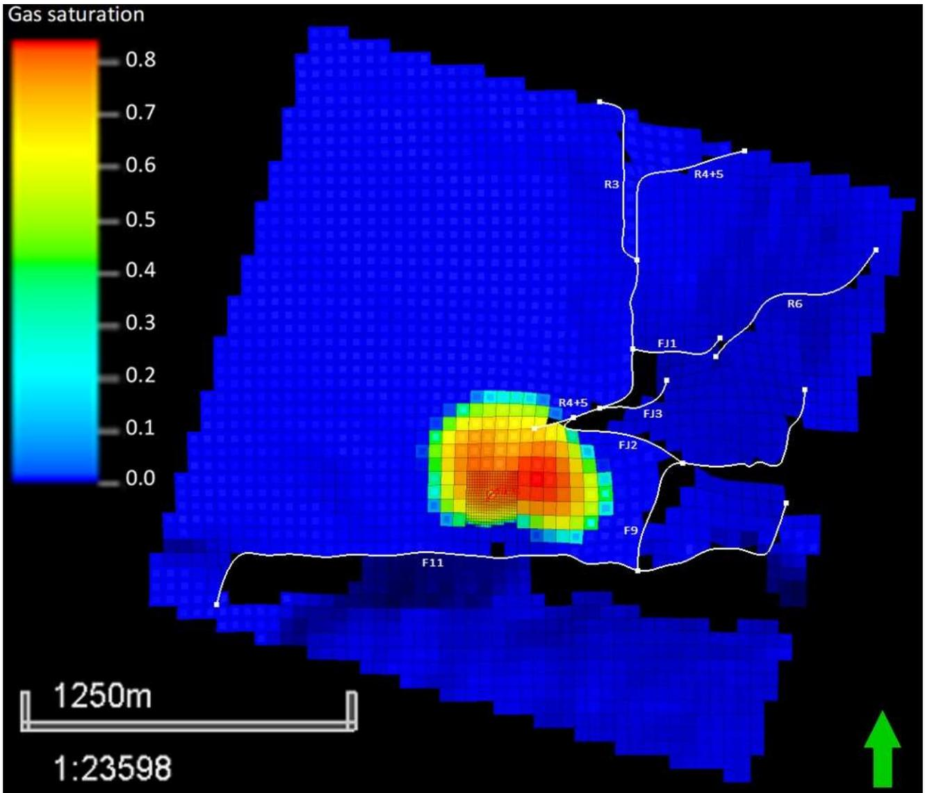
**Figure 19.** Location of faults in Sopeña Formation and migration distance of CO<sub>2</sub> plume from the injection well in 200 years of gas injection in a non-sealing scenario.
