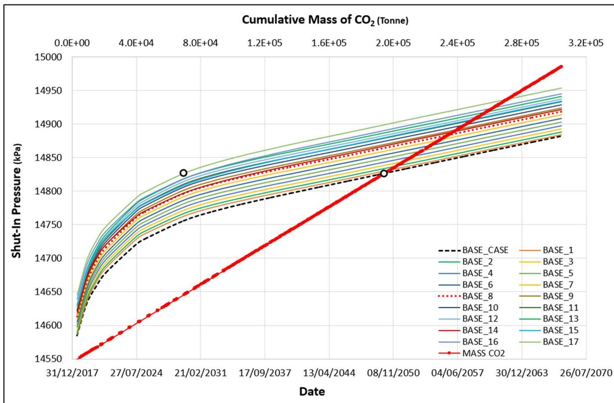
**Figure 11.** Reservoir shut-in pressure versus the cumulative injected mass of CO<sub>2</sub> for a similar time period. The heterogeneity of the simulated models based on the variation in matrix permeability.
