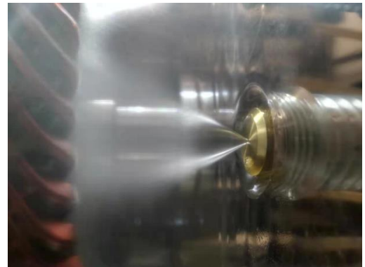
Fig. 9. Oil spray testing for case I with 50mm distance between the nozzle and the target surface
