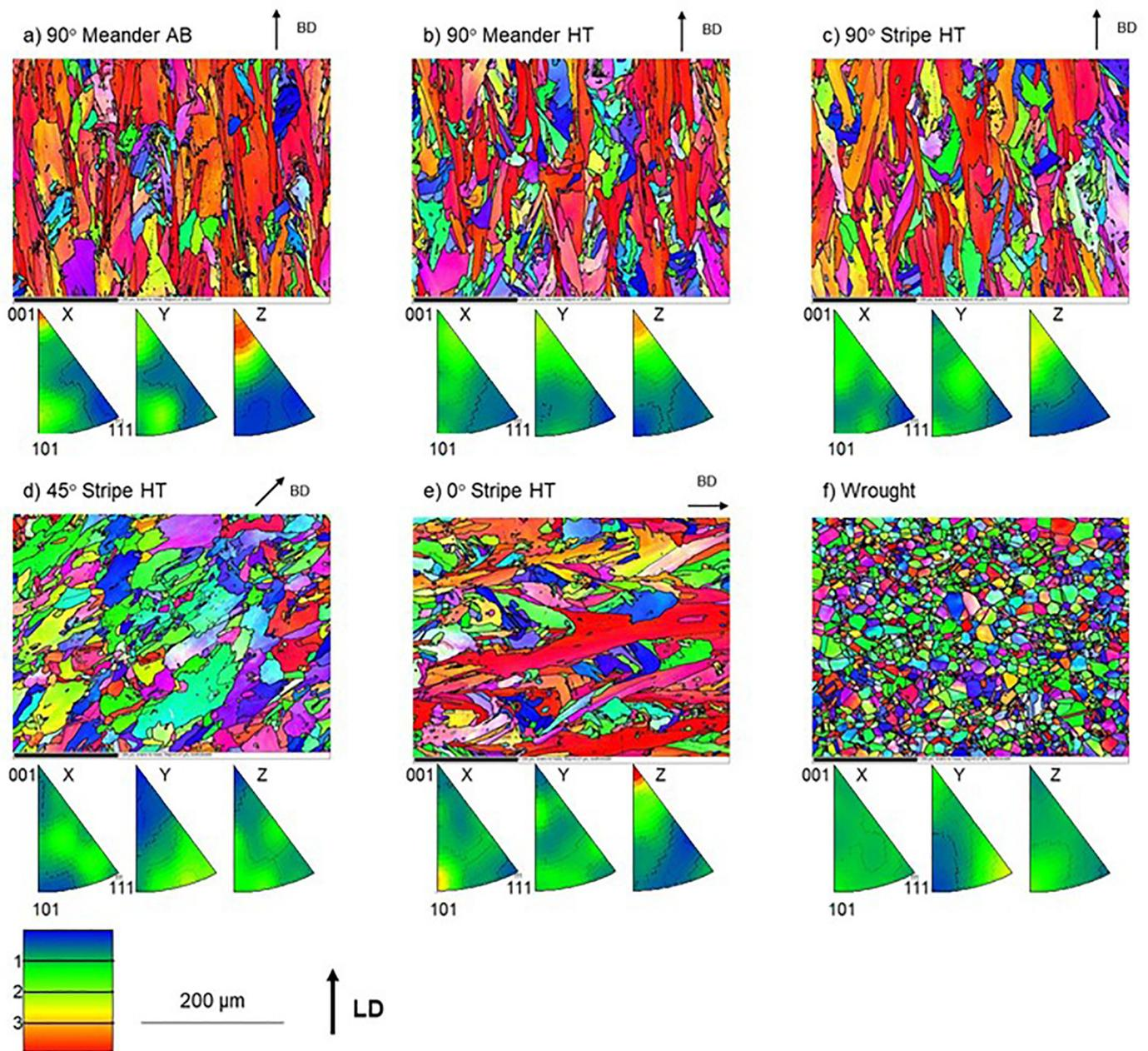
**Fig. 4.** EBSD maps and Inverse Pole Figures for a) 90° Meander AB specimens; Heat treated b) 90° Meander HT; c) 90° Stripe HT; d) 45° specimens; e) 0° Stripe HT and f) Wrought alloy 718. All images oriented with respect to the Loading Direction (LD), with the Build Direction (BD) indicated. Most LPBF specimen had a 001 texture parallel to their build direction. It is also clear that heat treatment reduced the texture and that Stripe specimen had less texture than their Meander counterpart.
