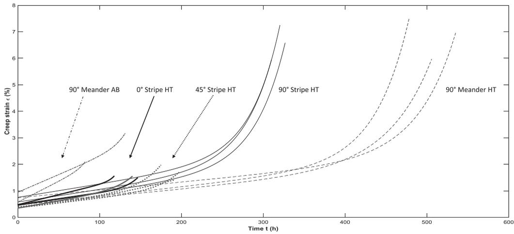
Fig. 5. Creep curves for the different test cases, showing the clear differences in creep performance with regards to orientation, heat treatment and scan strategy. This also shows the differences in tertiary creep for the different specimens.
