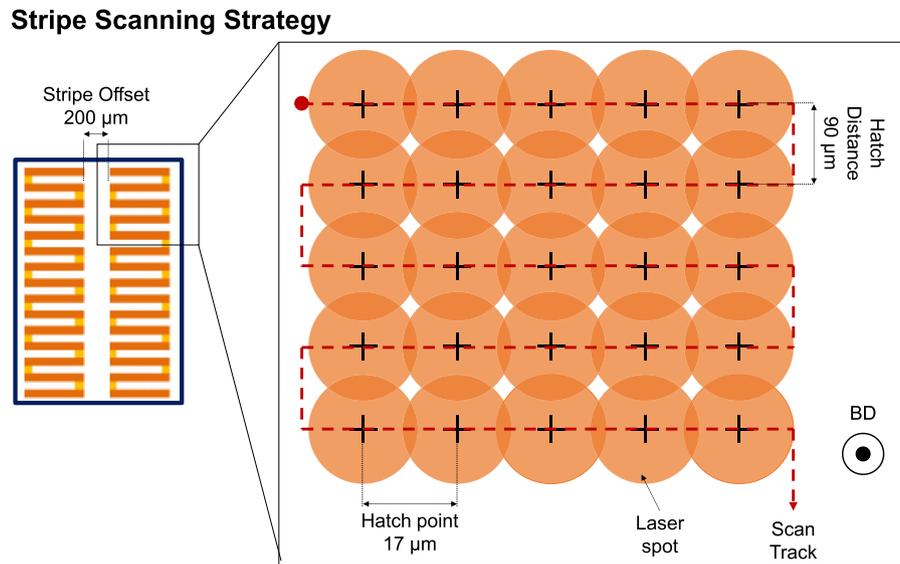
Fig. 2. Schematic representation of the Stripe scanning strategy showing the different parameters used. With the Build Direction (BD) indicated.
