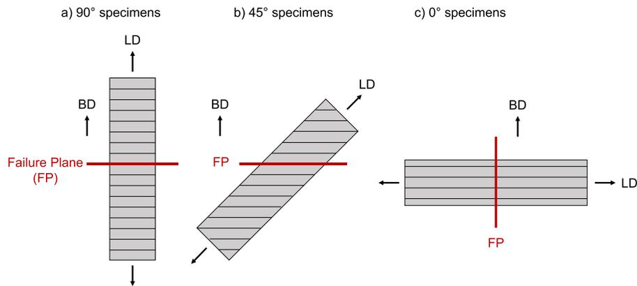
**Fig. 7.** Schematic representation of the failure planes of the different test cases, with respect to specimens' layers, build direction (BD) and with the Loading Direction (LD) shown. This shows that the stress state of the specimen also influenced their modes of failure.
