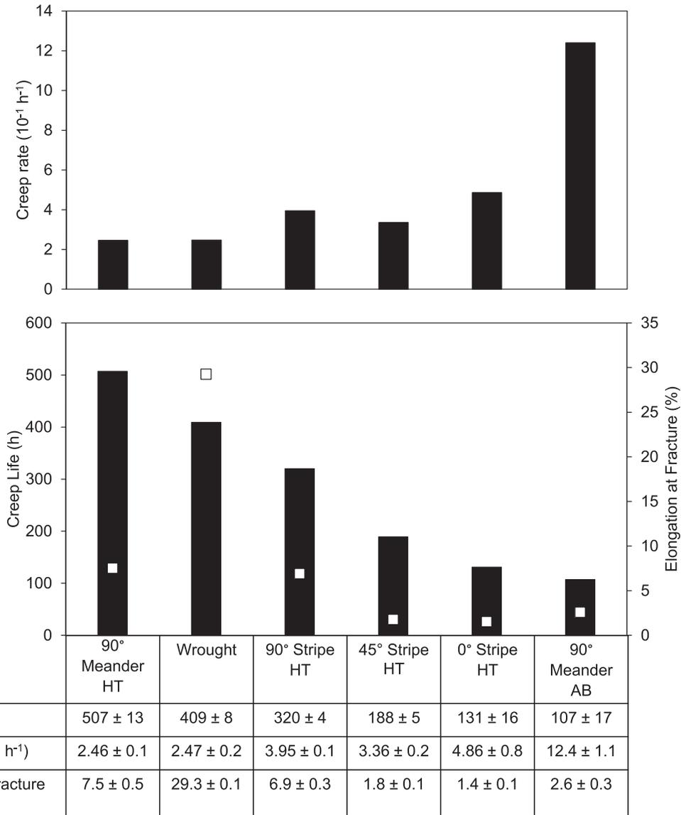
Fig. 6. Summary table and graph of the creep rate, elongation at fracture and creep life for all of the test cases, in order of decreasing creep life.
