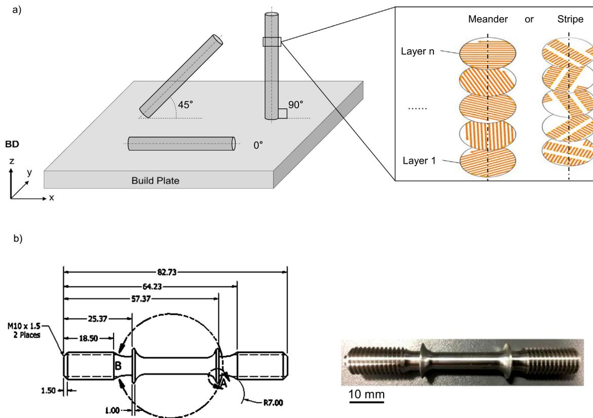
Fig. 1. Specimen overview: a) the different parameters investigated: Orientation and scan strategy; b) ASTM E8/E8M [20] uniaxial specimen after turning and grinding. With the Build Direction (BD) indicated.
