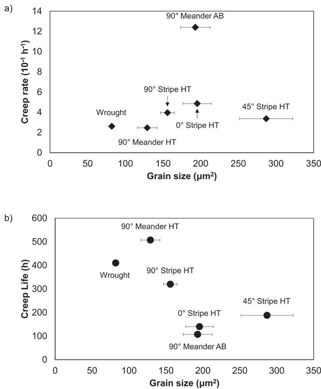
**Fig. 11.** Relationship between the grain size and a) the creep rate and b) the creep life for the different test cases.
