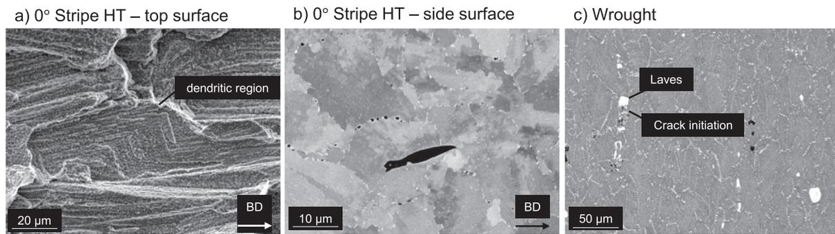
**Fig. 9.** SEM images of a) Trans-dendritic failure surface indicator in 0° Stripe HT specimen; b) Transgranular crack in 0° Stripe HT specimens and c) crack initiation at the Laves phase in Wrought specimens. All images oriented with respect to the loading direction, with the Build Direction (BD) indicated.
