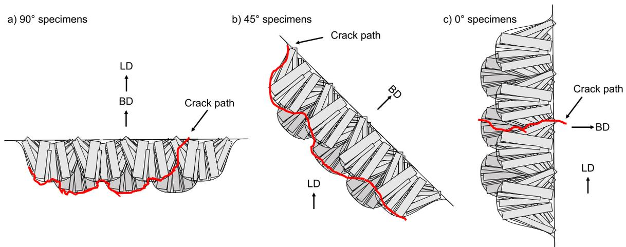
**Fig. 12.** Crack path for a) 90° specimens, where intergranular cracking occurred with some cleavage steps; b) 45° Stripe HT specimens where the intergranular cracking caused grain boundaries decohesion and sliding; and c) 0° Stripe HT specimens where Quasi-Cleavage occurred. All images oriented with respect to the Loading Direction (LD), with the Build Direction (BD) indicated.
