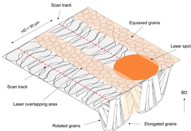
**Fig. 13.** Melt pool and grain formation schematic, showing the columnar and equiaxed grains. With the Build Direction (BD) and Hatch Distance (HD) indicated.
