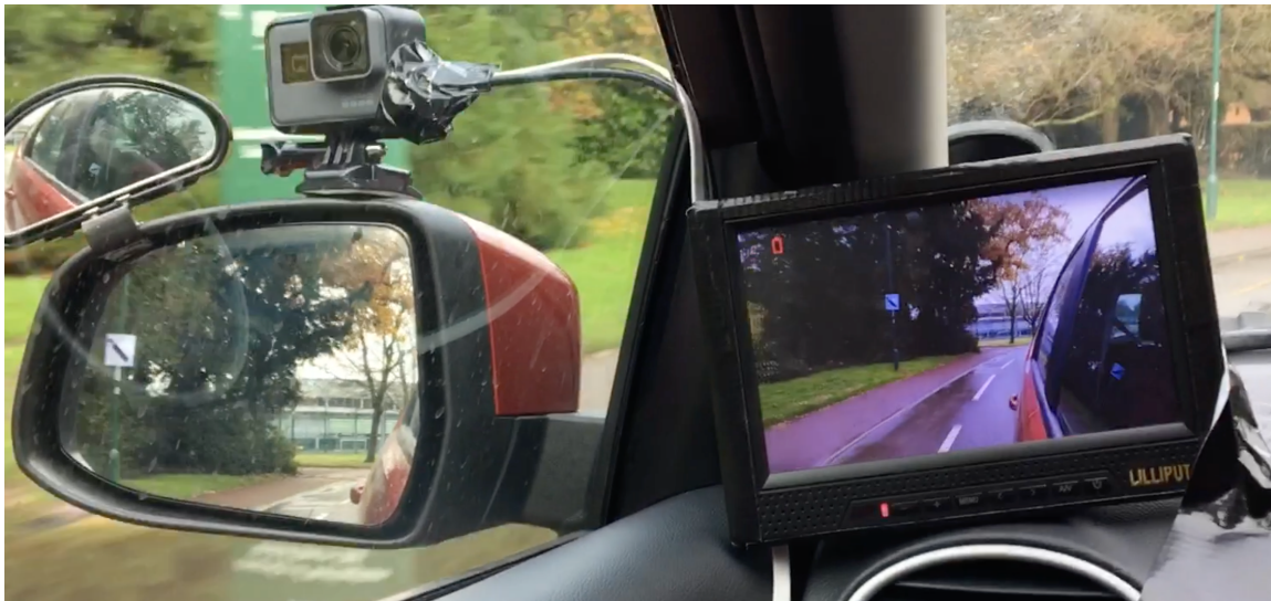
Figure 1: Experimental setup showing conventional reflective mirror and internal digital mirror connected to GoPro camera mounted on external mirror. Note: blind spot mirror provided for experimenter who drove the vehicle.
