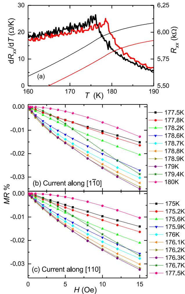
**Figure 2.** Electrical resistance versus temperature and applied magnetic field around  $T_C$ . **(a)** Resistance  $R_{xx}$  (thin lines) and its derivative  $dR_{xx}/dT$  (thick lines) versus temperature  $T$ , for Hall bar structures with current along  $[1\bar{1}0]$  (red) and  $[110]$  (black). **(b, c)** Magnetoresistance curves for **(b)** the  $[1\bar{1}0]$  and **(c)** the  $[110]$  oriented Hall bars, with magnetic field applied along the  $[1\bar{1}0]$  axis in both cases.
