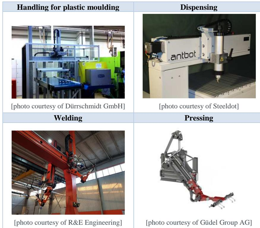
**Figure 7.2-7** Examples of applications of Cartesian robots. Image rights: Dürrshmidt GmbH, Steel dot, R&E Engineering, Güdel Group AG.
