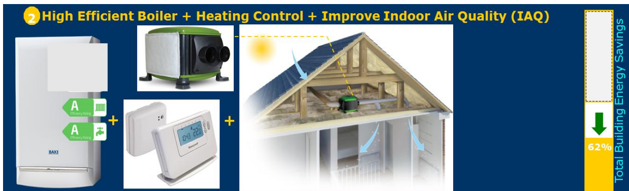
Figure 9: High efficient boiler, heating control, and Positive Pressure Mechanical Ventilation System (PPMVS)
