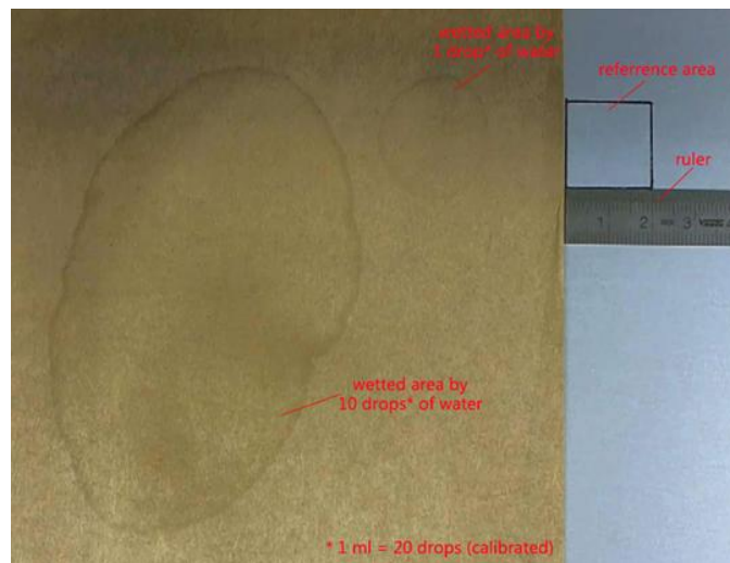
Figure 3: Kraft paper wetted area contrasting to the reference area
