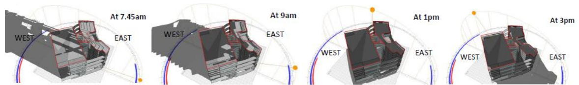
Figure 6: Daylight entering Interior at Different Time of the Day during Summer Solstice. Source: All Models by Author.
