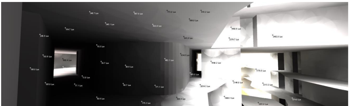
Figure 6: Under-lit corridors on Level B3, B2 and B1
