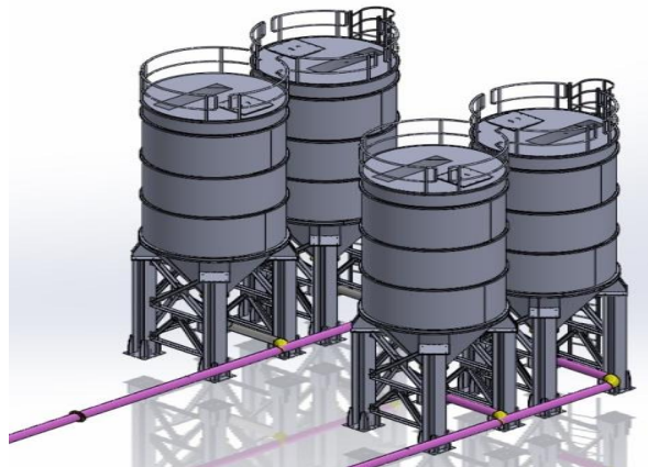
Figure 9: Conceptual model of Bio-Diesel transesterification silos
