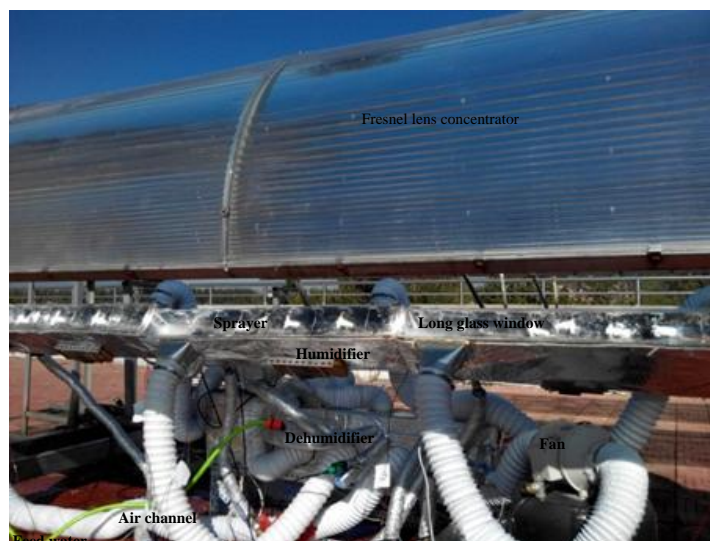
Figure 4: A photograph of the experimental set-up with insulation.
