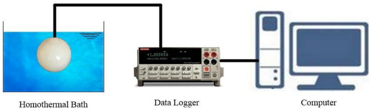
Figure 3: Schematic of experimental set-up
