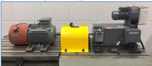
Fig. 22. Test rig: 15kW SynRel motor (left hand side) and 40kW induction machine used as a load (right hand side).
