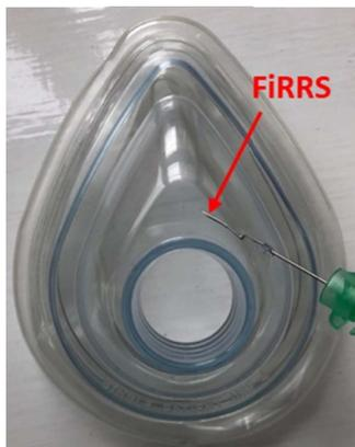
**Figure 3.** Anaesthetic mask with needle containing optical fibre inserted and used in part 2 of this research work.
