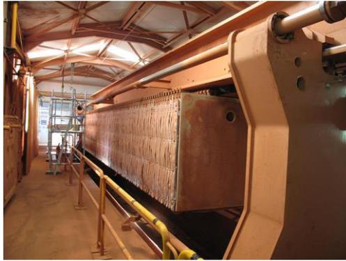
Figure 4. Plate and frame filter press, Gardanne, France [44].
