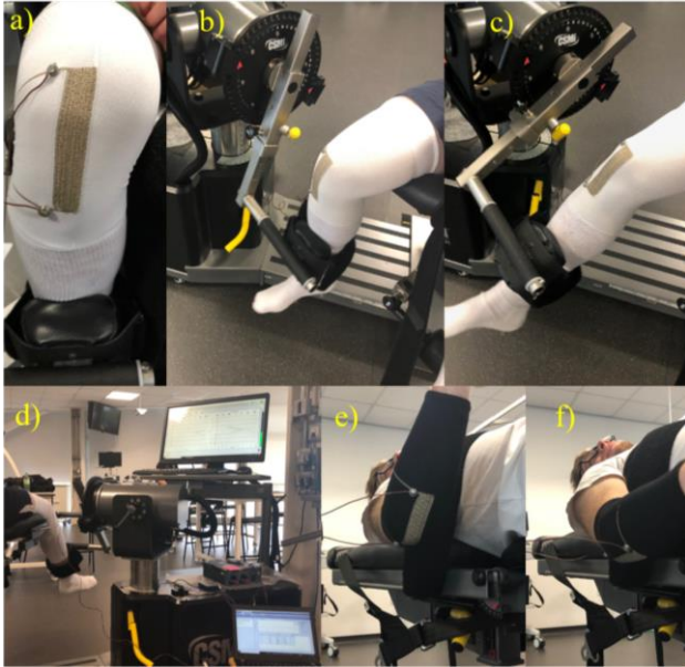
Figure 1 a) Close-up of the knitted sensor in the knee sleeve b) Knee sleeve in flexion c) Knee sleeve in extension d) Experimental set-up e) Elbow sleeve in flexion f) Elbow sleeve in extension
