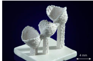
Figure 18: Dental restoration bridges produced by dLS of Al_2O_3-ZrO_2 showing the potential of the process for manufacturing complex parts in a single step, but with a very poor surface finish [311].
