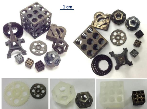
Figure 16: Examples of SiC ceramic parts produced by STL of preceramic polymer (top). Comparison of as-printed and pyrolysed/sintered samples (bottom).
