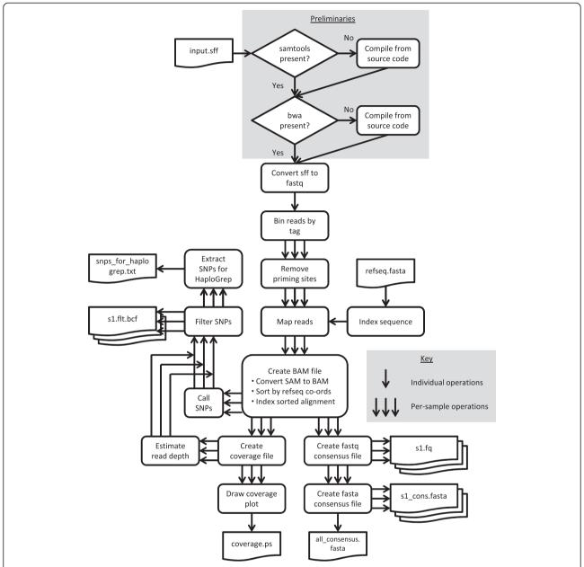
**Figure 3 Steps in the bioinformatics pipeline.** The pipeline automatically converts a single .sff input file from a 454 run containing the raw sequencing data for one or more individuals into a variety of useful output files, notably including per-individual consensus sequence and coverage plot files. To simplify usage it begins by detecting whether the necessary C programs have been installed, and automatically compiling bundled versions if not, before proceeding to the bioinformatics steps.
