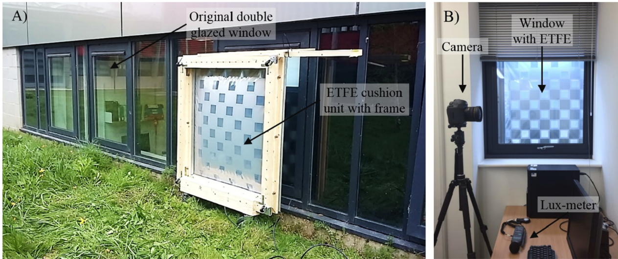
Fig. 6. External view of the building façade showing the installed ETFE cushion mock-up with the switchable sample DSF 3 (A). Interior view of the office space showing the camera in the view position for the 360° stereographic imaging (B).
