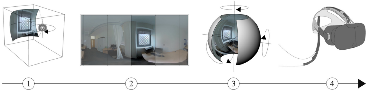
Fig. 7. Process of VR image generation, 1. HDRI photography of test room, 2. Stitching of images, 3. Post-processing and projection of images to spherical geometry, 4. Projection of imagery to VR headset as a stereoscopic environment.
