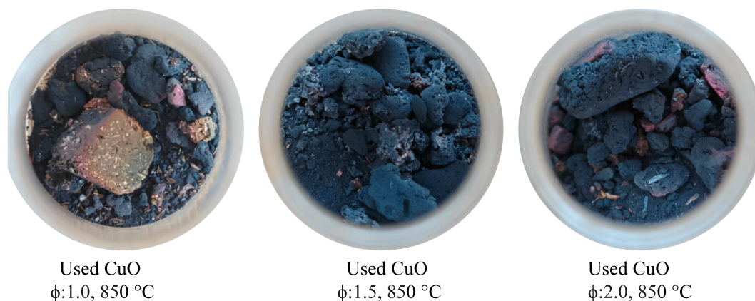
Fig. 8. Visual images of CuO (Inoxia) used in the combustion of biochar at 850 °C under stoichiometric ratio of \phi = 1.0, 1.5 , and 2.0 .
