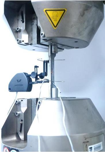
(b) Corner coupon test setup
