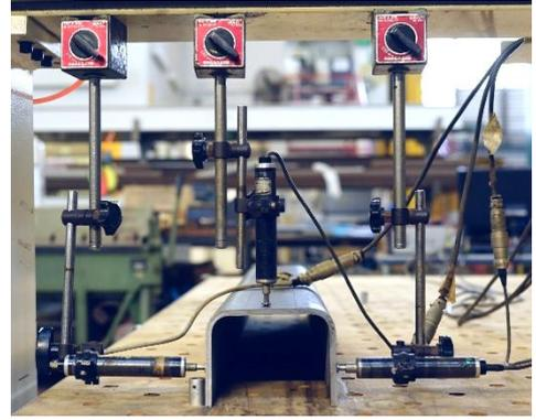
(b) Channel section stub column specimen C 120×90×6
