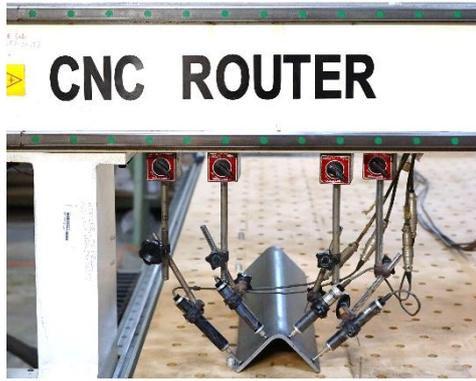
(a) Angle section stub column specimen A 60×6
