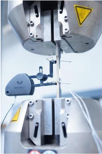
(a) Flat coupon test setup
