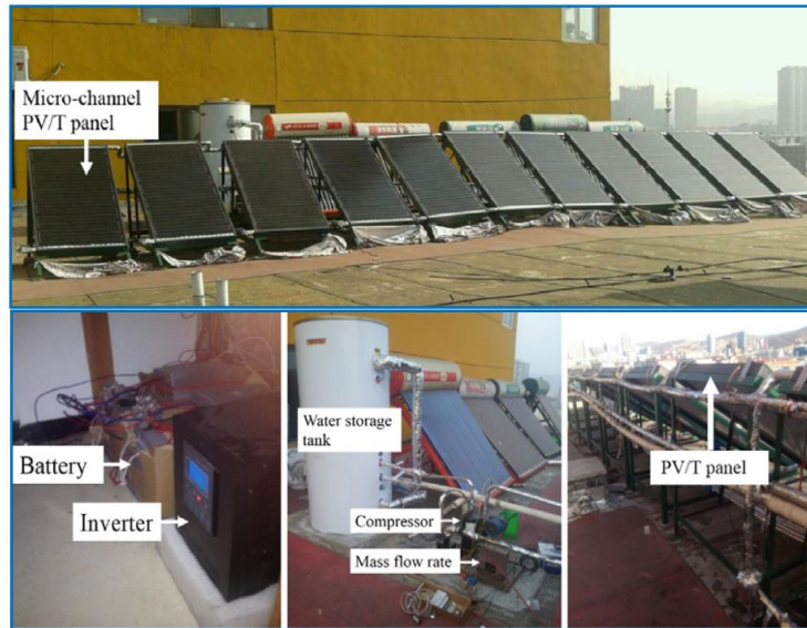
Fig. 40. Photos of the experimental rigs [68, 69]
