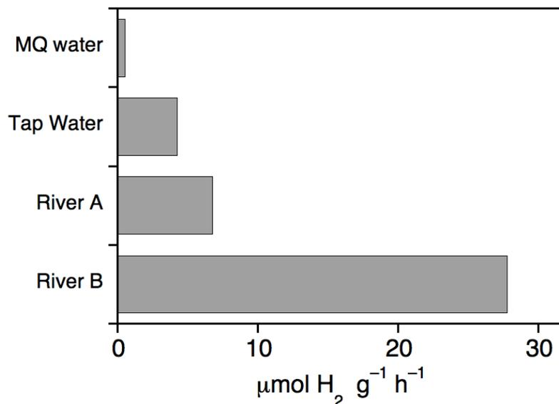
Figure 3: Hydrogen generation from different sources of water under solar simulated radiation. In this case MQ water is pure water from a Milli-Q system with 18.2 M $\Omega$  resistance. River A (Quebec) and river B (Ontario-Quebec border).
