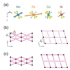
**Figure 9.** (a) Schematic of the ordered magnetic moments of Mn<sup>2+</sup>, Fe<sup>2+</sup>, Co<sup>2+</sup> and Ni<sup>2+</sup> in *M*(NCS)<sub>2</sub> (N atoms in grey-blue, S in yellow). The magnetic lattice adopted by Mn(NCS)<sub>2</sub>, Fe(NCS)<sub>2</sub> and Co(NCS)<sub>2</sub> is shown in (b), whilst (c) shows the magnetic lattice of Ni(NCS)<sub>2</sub>. Filled and empty circles denote collinear moments with opposite spatial orientations.
