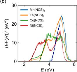
**Figure 5.** (a) Diffuse reflectance spectra for  $M(NCS)_2$  (M = Mn, Fe, Co, Ni). (b) Tauc plots of the diffuse reflectance data: extrapolation of the data to  $(F(R)hv)^2 = 0$  (indicated by the dashed line) yields the band gap for each material.
