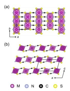
**Figure 1. (a)** Projection of a  $(2\times2\times1)$  supercell of  $M(NCS)_2$  (M=Mn, Fe, Co, Ni) down the c axis, highlighting the layers of edge-sharing  $[M^{2+}N_2S_4]$  octahedra. **(b)** Projection of a  $(2\times1\times2)$  supercell of  $M(NCS)_2$  down the b axis, showing the stacking of layers.
