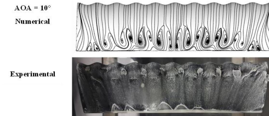
Fig. 16: Surface streamline visualization numerical and experimental for AOA 10°.
