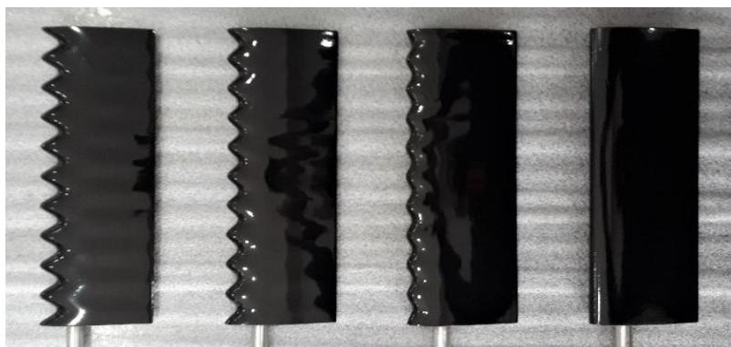
Fig. 4: Designed wings – 'A12 $\lambda$ 25', 'A8 $\lambda$ 25', 'A4 $\lambda$ 25', and 'Baseline' from left to right.
