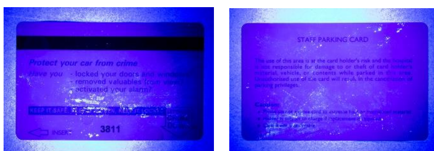
Figure 1: Dye transferred onto clean ticket. Figure shows the first ticket inserted and retrieved from the machine following the insertion of a contaminated ticket, front & rear view.
