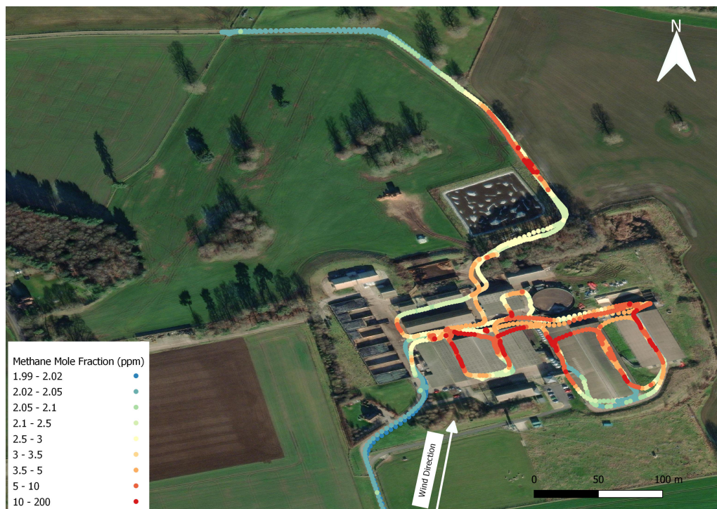
Figure 6. Mapping a UK dairy farm for methane emissions. Wind from south-south west (lower left). Air around large cow-filled barns in lower centre of map has very high methane. Large manure holding lagoon of figure 7, covered by membrane and water also has high values. Note scale bar (100 m). (study by A Alshalan).
