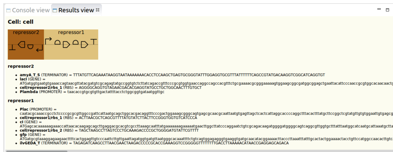
Figure 5. Biocompiler result for the toggle switch specification. Sequence information of promoters, coding regions and terminators is drawn from several online repositories (here the iGem parts registry), and ribosome binding sites are automatically calculated using Salis' ribosome binding site calculator.
