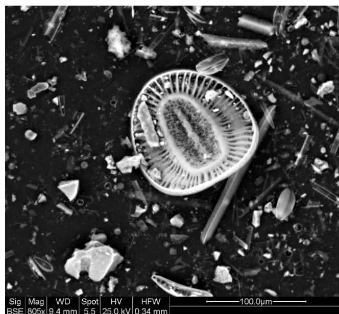
Fig. 2. SEM image of Campylodiscus clypeus highlighting the difficulties of producing a contaminant-free diatom sample when minerogenic matter attaches to diatoms. Mass balance corrections can be used to correct for the effect of this on \delta^{18}\text{O}_{\text{diatom}} data.
