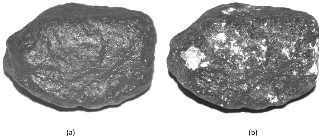
Fig. 1. Images of ballast particles subjected to wear: before (a) and after (b).
