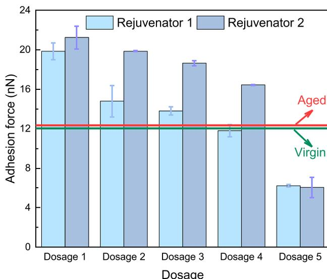
Fig. 11. Adhesion properties of rejuvenated bitumen.
