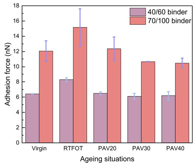
Fig. 10. Adhesion properties of bitumen in terms of ageing.
