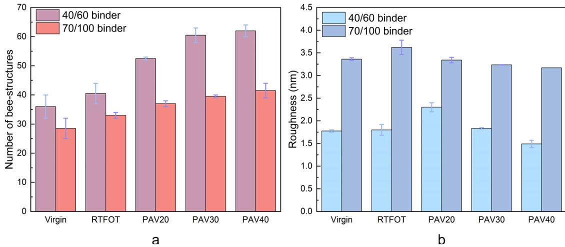
Fig. 4. Quantitative characteristics of micromorphology of bitumen in terms of ageing (a) Bee-structures and (b) Roughness.
