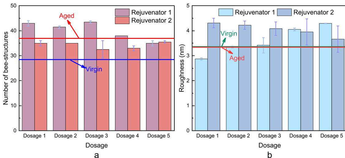
Fig. 6. Quantitative characteristics of micromorphology of bitumen in terms of rejuvenation (a) Bee-structures and (b) Roughness.
