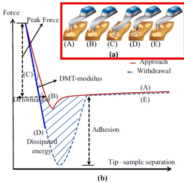
**Fig. 1.** Working principle of AFM (sourced from [45]).
