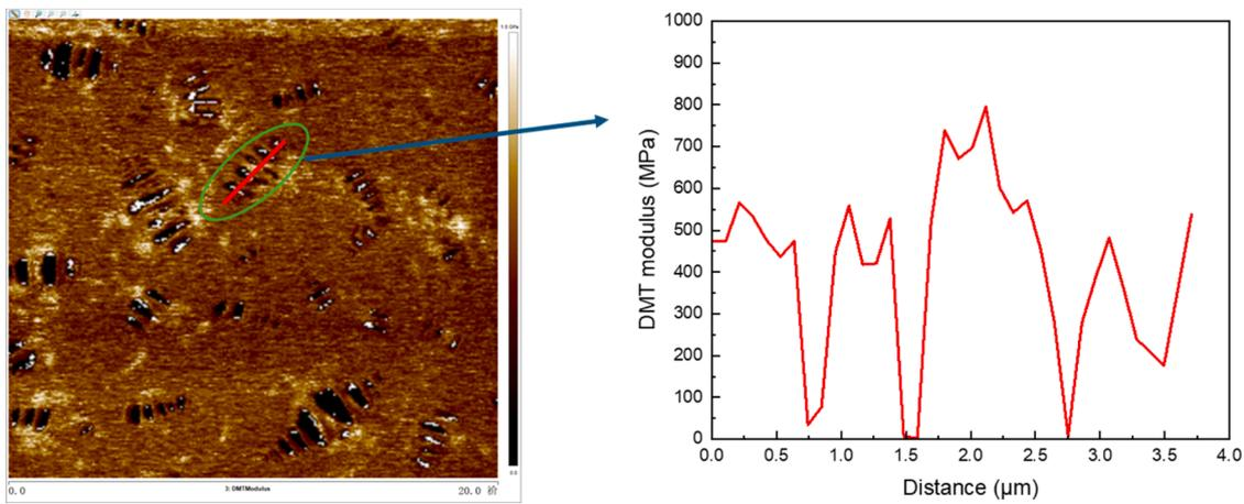
Fig. 7. 2D DMT modulus image (left) and DMT modulus mapping (right).
