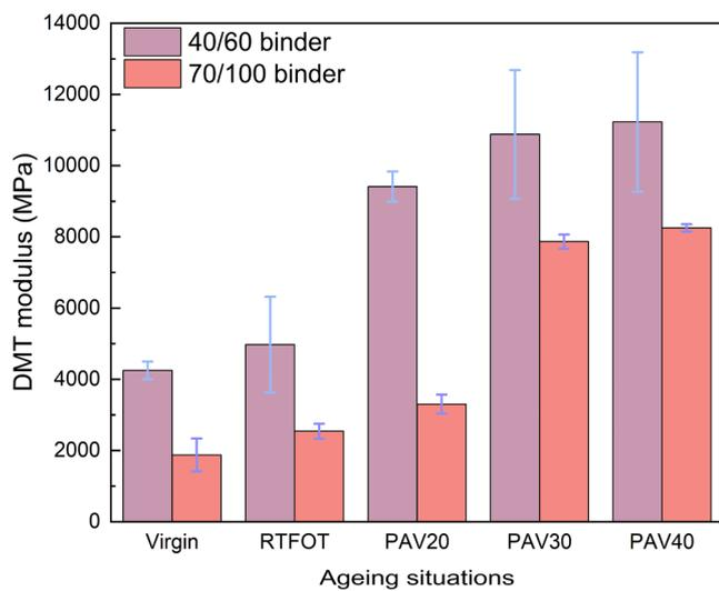
Fig. 8. DMT modulus of bitumen with different ageing levels.
