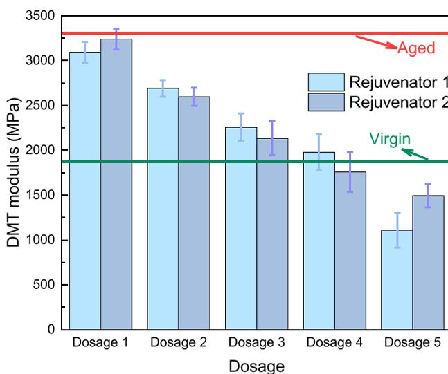
Fig. 9. DMT modulus of rejuvenated bitumen using different rejuvenators.
