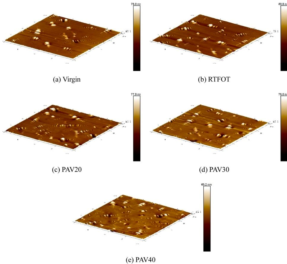
Fig. 3. 3D topography of bitumen with varying ageing levels.
