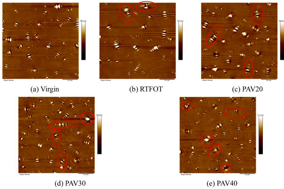
Fig. 2. 2D topography of bitumen with varying ageing levels.
