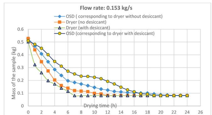
Fig. 8. The variation of the sample’s mass over time in different drying modes. [51].
