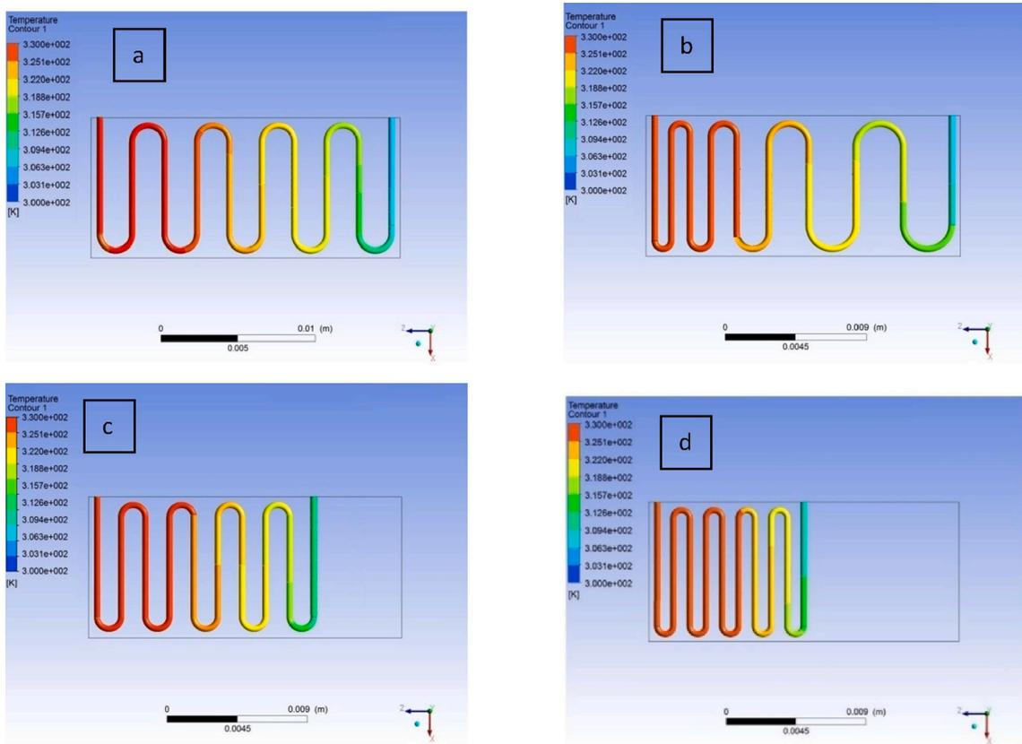
Fig. 6. Temperature readings for various distributions of PCM tubes along the Flat Plate Collector (FPC) at 9:00, considering an airflow rate of 0.025 kg/s [49].
