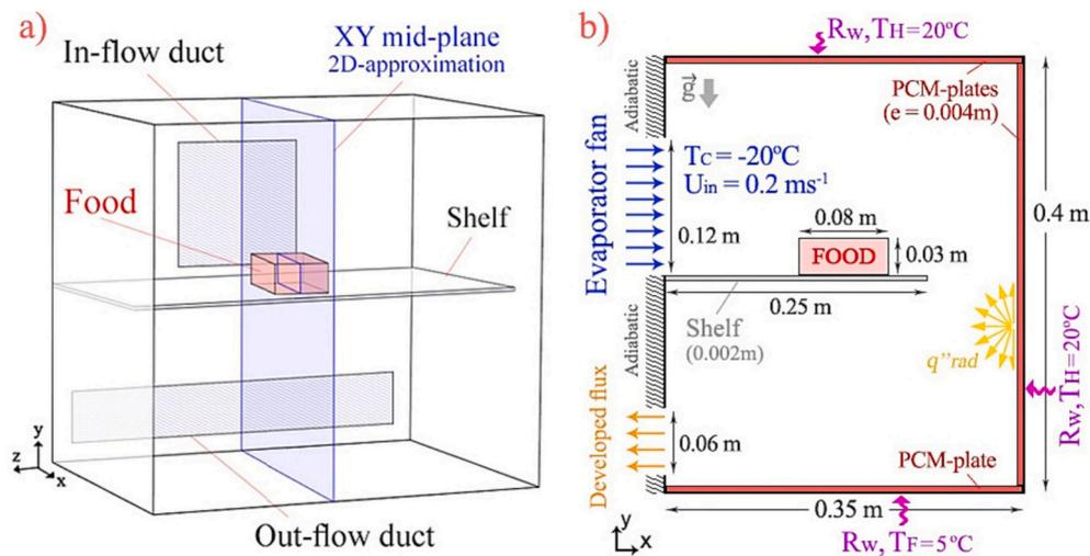
Fig. 14. Physical model of the convective freezer WPCM plates: (a) three-dimensional view; (b) 2D study domain. [97].
