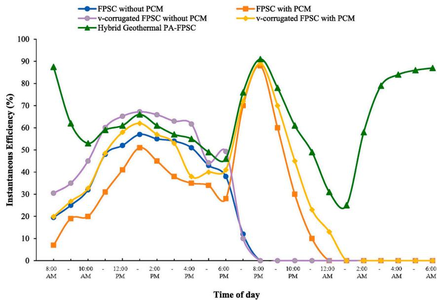
Fig. 10. A comparison of the real-time efficiencies of various types of FPSC with hybrid geothermal PA-FPSC [75].
