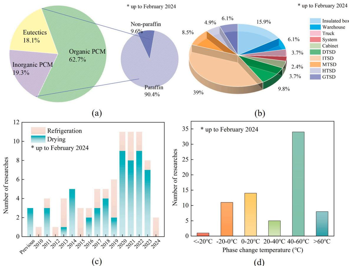
Fig. 4. Statistic of PCMs applications and properties employed in food storage process: (a) types of PCMs (b) PCMs applied in different devices (c) number of publications over the years (d) number of publications under different PCMs phase change temperature.
