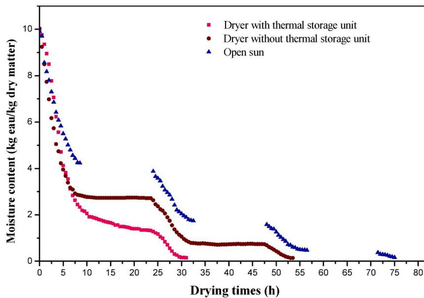
Fig. 11. Evolution of moisture content of red pepper in GTSD WPCM/WOPCM and open sun dryer with drying time [77]. (For interpretation of the references to color in this figure legend, the reader is referred to the web version of this article.)
