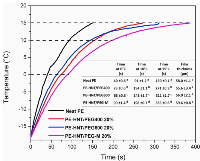
Fig. 13. Time-temperature profiles illustrating the thawing process from  $-18\text{ }^{\circ}\text{C}$  to room temperature for both neat PE film and PE-HNT/PEG nano-composite films. Tabulated data indicates the elapsed time for the frozen films to reach  $0\text{ }^{\circ}\text{C}$ ,  $10\text{ }^{\circ}\text{C}$ , and  $15\text{ }^{\circ}\text{C}$ , along with the thickness of the films. [86].
