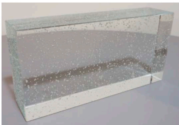
Figure 9. An untoughened crystal glass brick with sparsely suspended bubbles.
