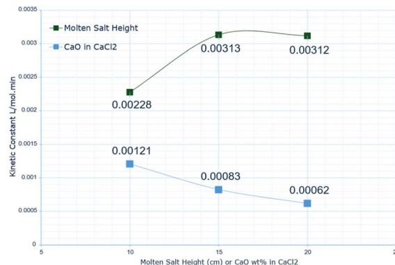
Fig. 10 Calculated kinetic constants for the molten salt and CaO wt% in CaCl 2 data.
