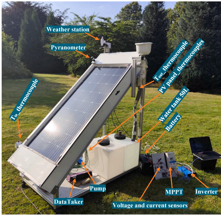
Fig. 2. Experimental set-up of closed-loop hydronic cooling of PV panel.
