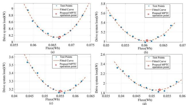
Fig. 9. Stator flux sweep test results with different load at 8000 r/min. (a) Torque260Nm. (b) Torque200Nm. (c) Torque140Nm. (d) Torque80Nm.
