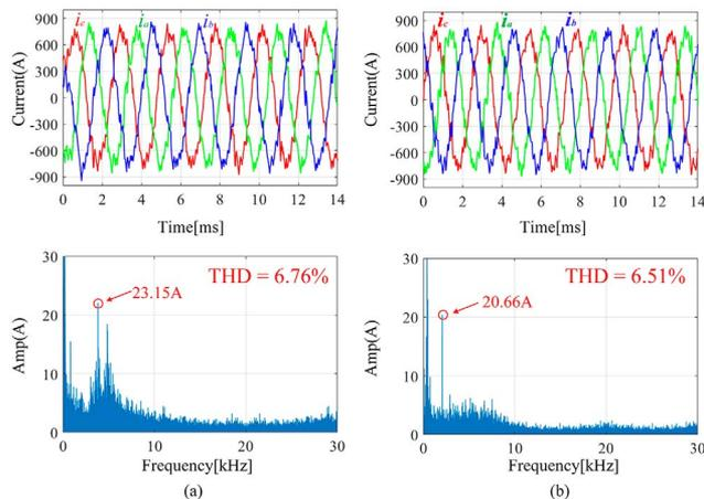
Fig. 10. Steady state phase currents waveform at full load, 5000 r/min. (a) Steady-state phase currents waveforms for MPTC+LM. (b) Steady-state phase currents waveforms for proposed MPTC.
