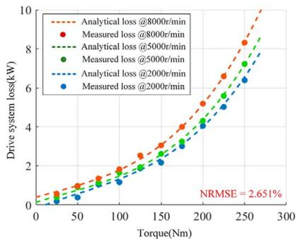
Fig. 8. Comparison of the PMSM drive system loss with proposed loss model estimation and measurement results.
