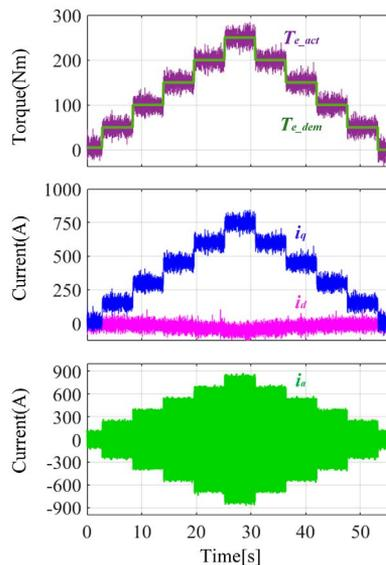
Fig. 13. Measured results of the proposed MPTC strategy at base speed with various load conditions.
