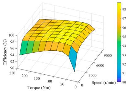
Fig. 15. Drive system efficiency with proposed MPTC strategy under various conditions.
