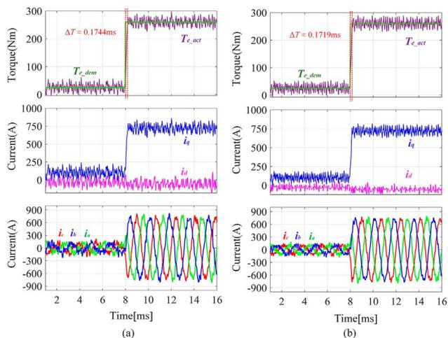
Fig. 12. Step load from 10% of rated load to 100% at base speed. (a) MPTC+LMC. (b) Proposed MPTC.
