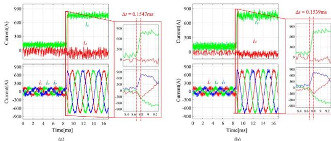
Fig. 5. Torque dynamic response as the torque step from 20% to 100%. (a) MPTC+LMC. (b) Proposed MPTC.
