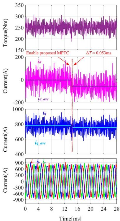
Fig. 11. Minimization loss tracking test of proposed MPTC strategy at rated load, base speed.
