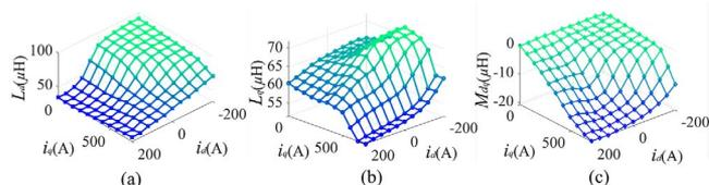
Fig. 7. Stator inductances under various  $dq$ -axis current conditions. (a)  $d$ -axis inductance. (b)  $q$ -axis inductance. (c)  $dq$ -axis mutual inductance.
