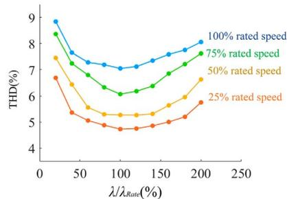
Fig. 6. THD versus weighting factor of nominal at different load.
