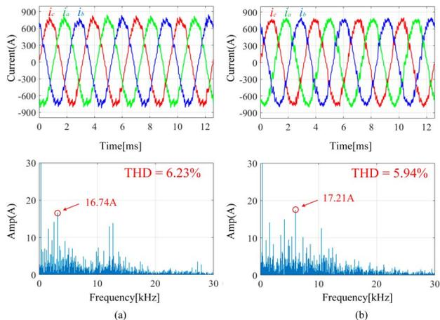
Fig. 4. Steady-state current waveforms and harmonic spectrum at 3000 rpm and 260 Nm. (a) Steady-state phase currents waveforms for MPTC+LMC. (b) Steady-state phase currents waveforms for proposed MPTC.
