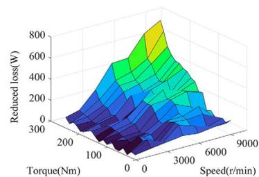
Fig. 14. Measured loss reduction of the proposed MPTC strategy compared with conventional MPTC+MTPA strategy.
