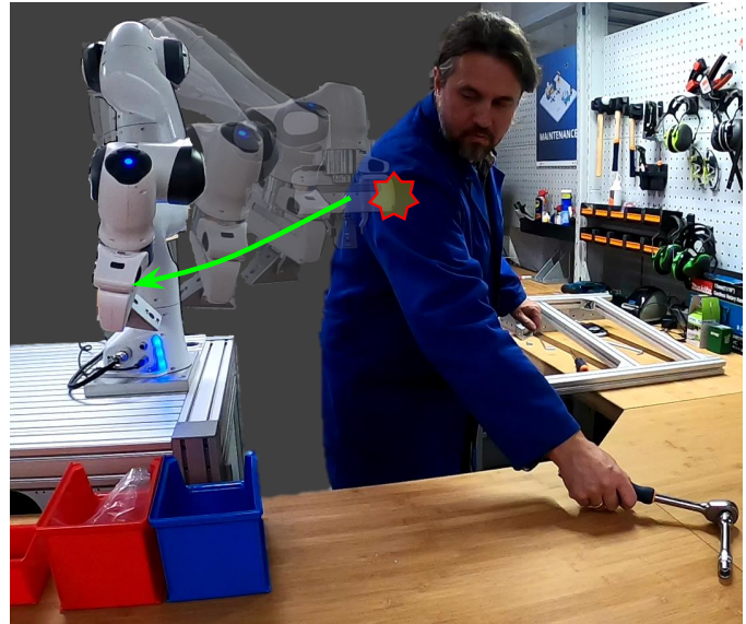
Figure 1. The abrupt movement of the human to grasp the tool results in an unavoidable collision in a close human-robot collaboration scenario. Consequently, a collision reflex has to be activated to ensure the safety of both the human and the robot.
