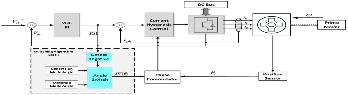
Fig. 8 Proposed improved controlled system solution for SRG load handling
