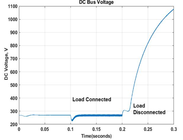
Fig. 7 DC Bus voltage failure when handling load
