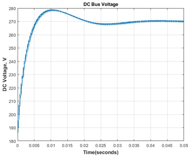
Fig. 12 DC Bus voltage with no load applied
