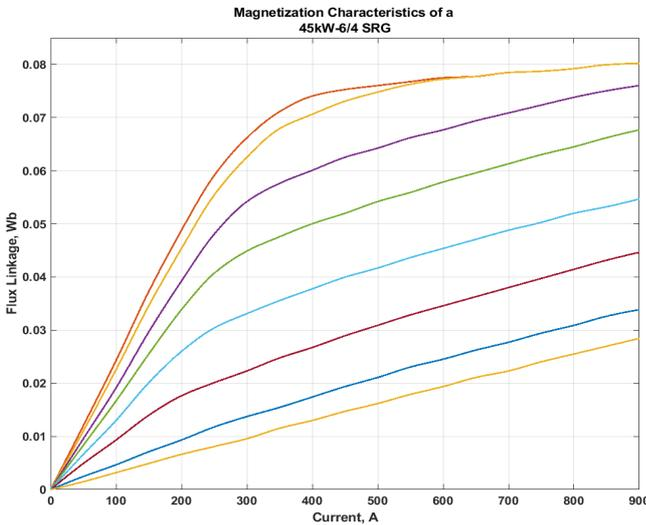
Fig. 3 Magnetization Characteristic of 45kW 6/4 SRG
