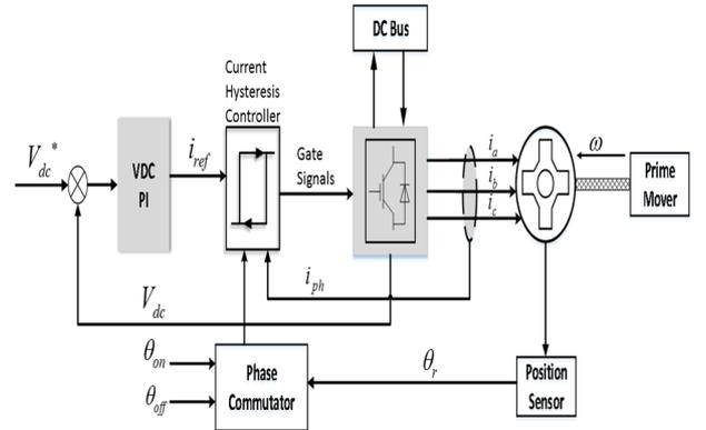
Fig. 4 A generic structure of SRG Drive System for aircraft application
