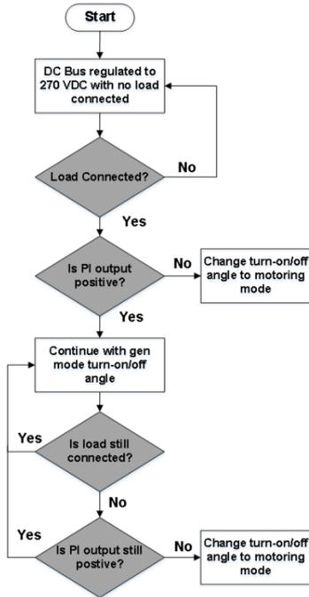
Fig. 9 Angle Switching Algorithm
