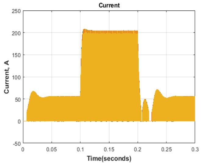
Fig. 13 Current behavior when load is applied ( $t=0.1s$ ) and disconnected ( $t=0.2s$ )
