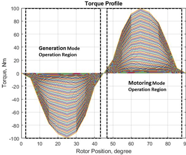
Fig. 6 Torque profile calculated using Eq.(4) and using magnetic properties from Fig. 3
