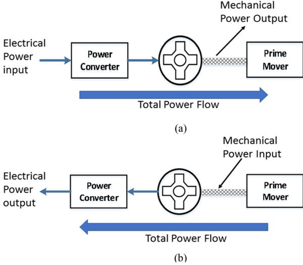
Fig. 2 Power conversion in (a) Motoring mode (b) Generation mode
