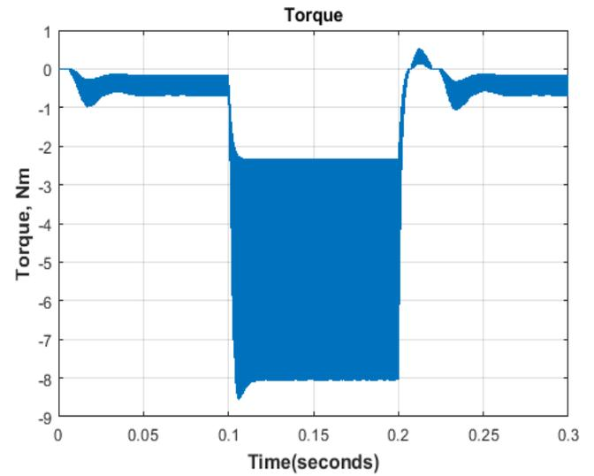
Fig. 14 Torque behavior when load is applied ( $t=0.1s$ ) and disconnected ( $t=0.2s$ )
