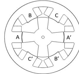
Fig. 1 Geometrical structure of a 3-phase 45kW 6/4 SRM
