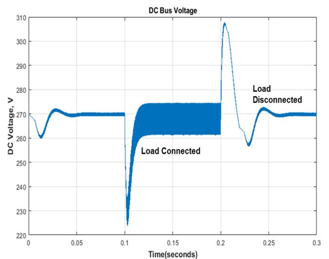
Fig. 15 DC Bus voltage with load applied at  $t=0.1s$  and disconnected at  $t=0.2s$ .
