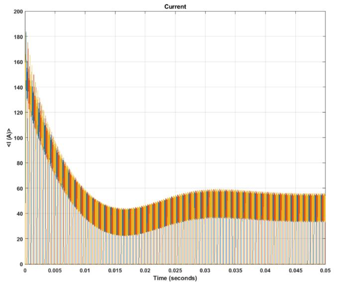
Fig. 10 Current behavior at stator with no load applied
