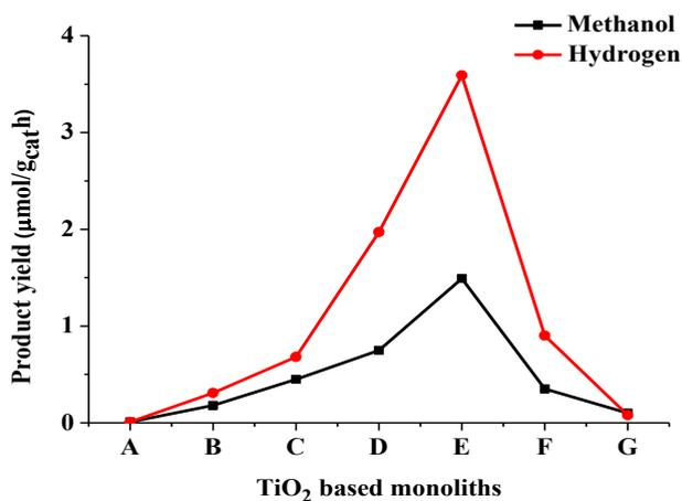
Fig. 1. Effect of Cr doping on TiO<sub>2</sub> based monoliths threaded with optical fibers for CO<sub>2</sub> photocatalytic reduction under visible light irradiation. ((A) TiO<sub>2</sub>, (B) 0.1wt% Cr-TiO<sub>2</sub> with no optical fibers, (C) 0.1wt% Cr-TiO<sub>2</sub>, (D) 0.5wt% Cr-TiO<sub>2</sub>, (E) 1wt% Cr-TiO<sub>2</sub>, (F) 1.5wt% Cr-TiO<sub>2</sub> and (G) 2wt% Cr-TiO<sub>2</sub>; C-G were tested with optical fibers)
