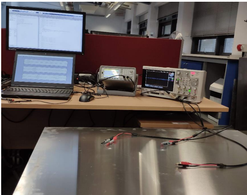
Fig. 9: Experimental suite used comprising a laptop, an arbitrary waveform generator, and an oscilloscope connected to the PZT transducers attached to the metallic specimen.
