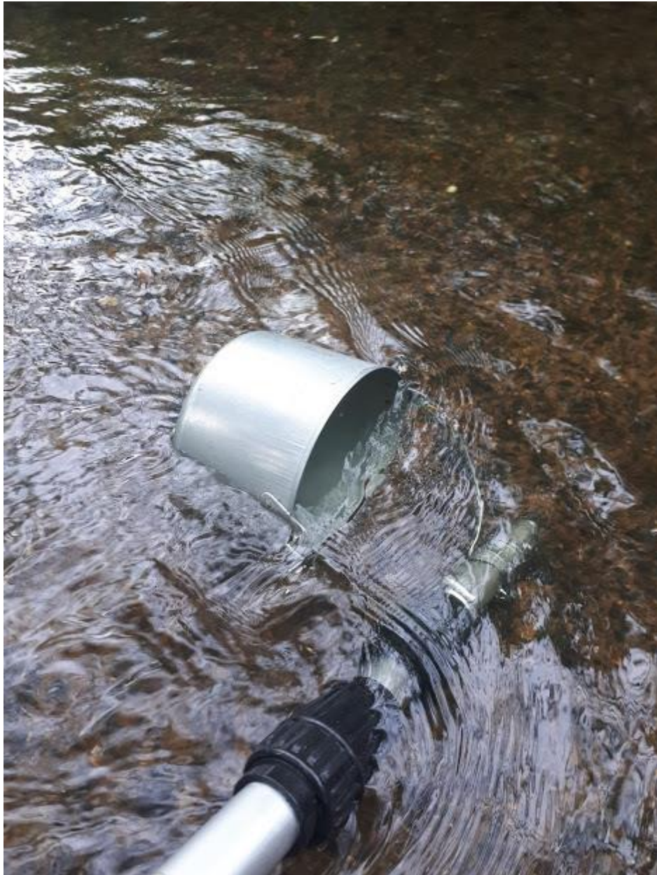
Figure S2: Photograph of sampling apparatus indicating the shallow nature of the some of the sampled sites. In the photograph the approximate water depth is 77.5 mm
