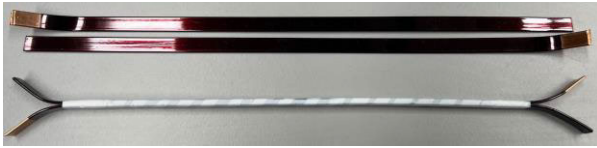
FIGURE 2. Illustration of edgewise insulated wires, displaying their condition prior to (top) and following (bottom) PTFE wrapping, representing the test sample.
