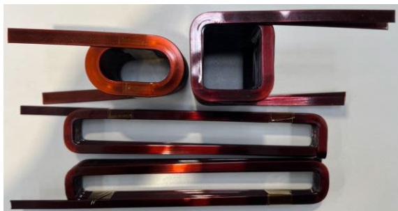
FIGURE 1. Depiction of coil windings fabricated using edgewise-insulated wires on the university of nottingham's production line.
