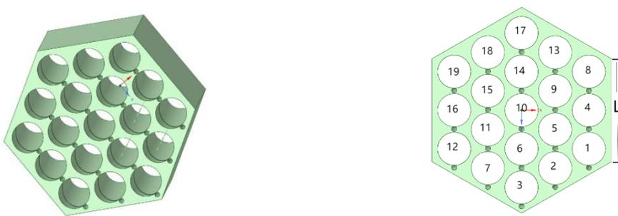
Figure 2.1: Computational fluid domain    Figure 2.2: Front view of the fluid domain
