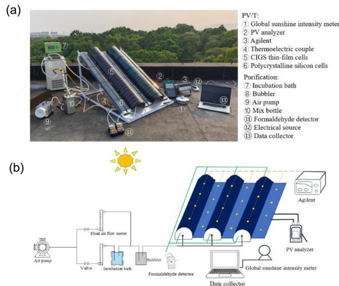
Figure 4: The PV-TC roof system: (a) Physical diagram (b) Schematic diagram
