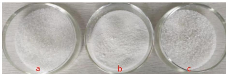
a) Silica      b) Anhydrous LiCl      c) Silica-LiCl composite
