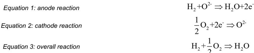
The Nernst potential represents the electromotive force ( $E_{\text{cell}}$ ) between the cathode and anode (Xingguo 2023). When current flows through the SOFC, the potential difference between the cathode and anode creates a resistance to the flowing current, such as
