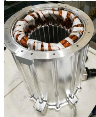
Fig. 1. Litz wire use within an aerospace generator.
