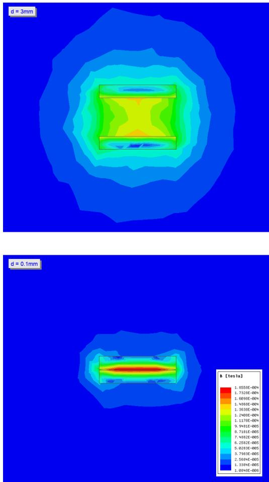
Figure 3: Simulated magnetic flux density in the vicinity of two conductors carrying opposing currents as the space between them is varied. Spacing between conductors in the diagram at the top is 3mm, whilst the spacing in the diagram at the bottom is 0.1mm. In both diagrams; current flows into the page in the upper conductor and out of the page in the lower conductor. Simulation undertaken using *Ansys Maxwell* with an excitation of 1A.
