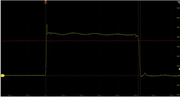
Figure 5: The half bridge under a double pulse test at 450V, 72A. Yellow trace is  $V_{ds}$  of switched device, red trace is the inductor current. Timebase is 100ns per division, vertical scale is 100V per division.
