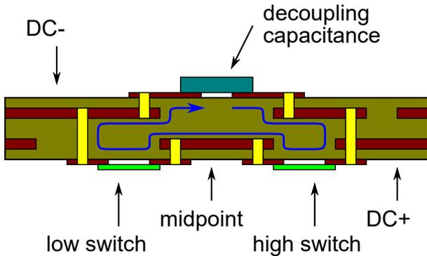
Figure 4: Cross section of the final half bridge PCB design. The commutation loop is indicated by the blue arrow. Copper areas are indicated in maroon. Vias are indicated in yellow. FR4 is indicated in olive. Diagram not to scale.
