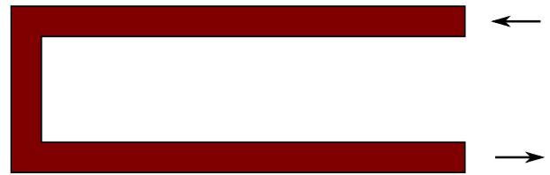
(a) Current carrying loop arranged in the plain of a single copper layer. Viewed from above.
