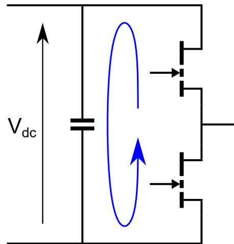
Figure 1: Diagram showing the typical arrangement of a half bridge. The commutation loop is indicated by the blue arrow.
