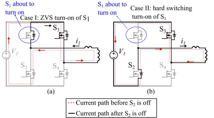
Fig. 6. Equivalent converter circuit during turn-off of semiconductor device  $S_2$  and turn-on of  $S_1$ : a) soft-switching and b) hard-switching turn-on.
