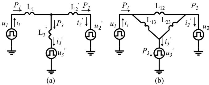
Fig. 3. a) Y- and b)  $\Delta$ -equivalent circuit model of TAB converter.
