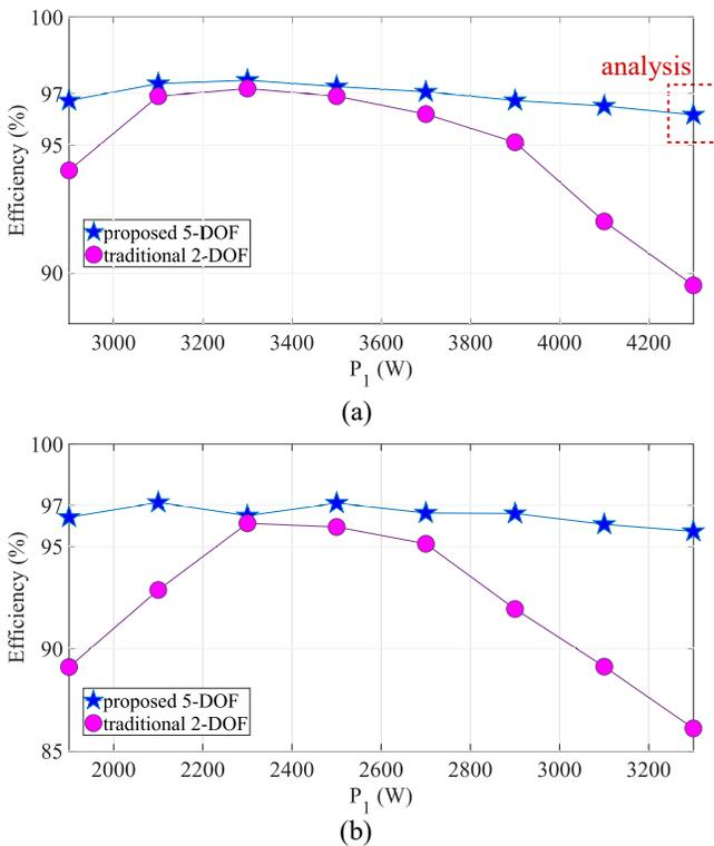
Fig. 14. Converter prototype efficiency for 5-DOF operation with the proposed total loss optimization scheme and the traditional 2-DOF modulation; a) simultaneous charging of HV and LV batteries from the grid (G2B) and b) individual HV battery charging from the grid and LV battery at zero average power (G2H).
