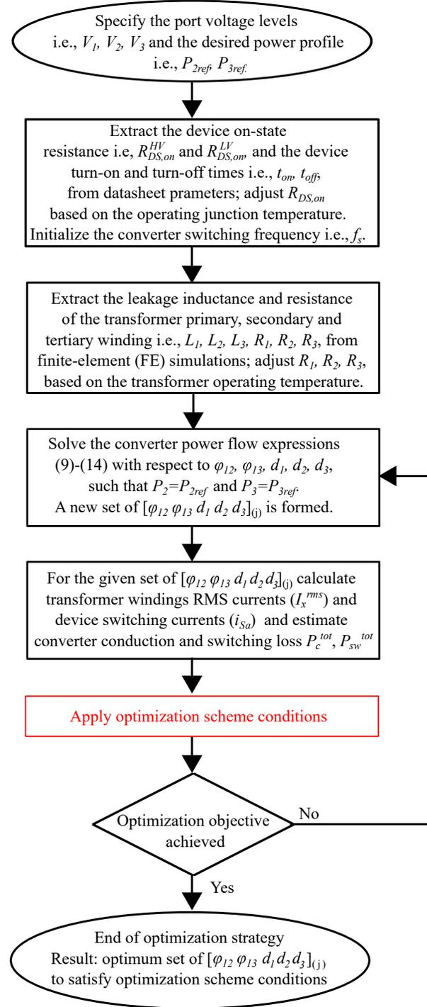
Fig. 7. Flowchart of the TAB converter optimization strategy.
