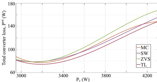
Fig. 10. Comparison of total converter loss for four different optimization schemes i.e., multi-current (MC) conduction loss, switching loss (SW), zero-voltage-switching (ZVS) and total loss (TL);  $V_{DC} = 325V$ ,  $V_{LV} = 48V$ ,  $P_3 = 1kW$ , while  $V_{HV}$ ,  $P_2$  vary from 1.9kW at 250V to 3.3kW at 420V.
