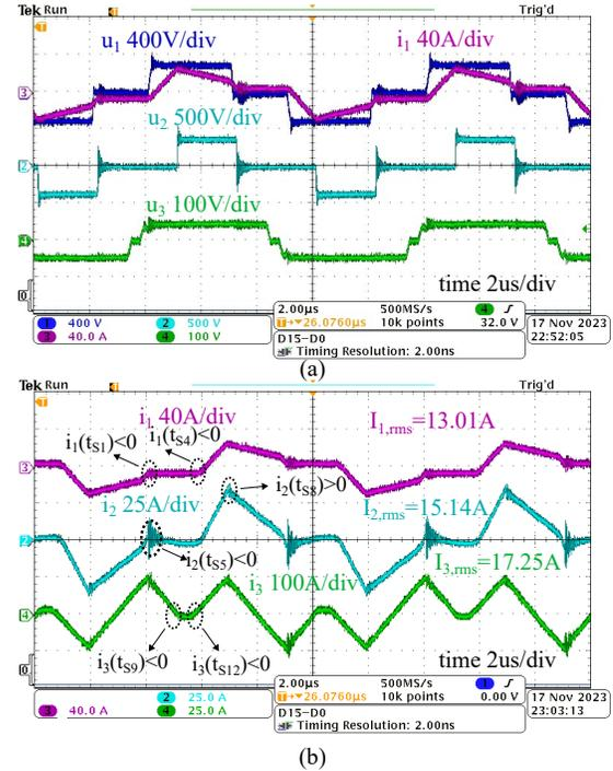
Fig. 13. Experimental TAB converter a) voltage and b) current waveforms for individual HV battery charging at nominal power levels i.e.,  $V_{DC} = 325V$ ,  $V_{HV} = 420V$ ,  $V_{LV} = 48V$ ,  $P_2 = 3.3kW$  and  $P_3 = 0W$ ; optimization based on the total loss optimization scheme with  $d_1 = 1.88$ ,  $d_2 = 1.41$ ,  $d_3 = 2.83$ ,  $\phi_{12} = 0.28$ ,  $\phi_{13} = 0.25$  (degrees-of-freedom are given in rad).
