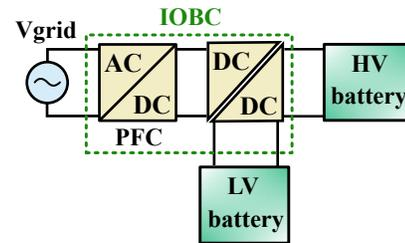
Fig. 1. Schematic diagram of an integrated OBC-APM charger.
