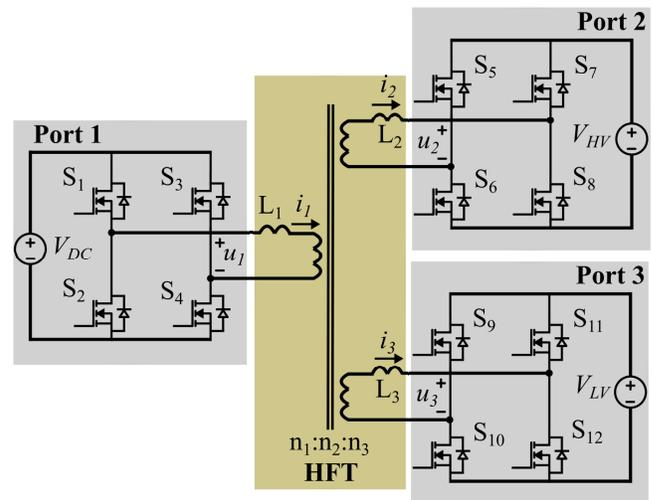
Fig. 2. Topology of the proposed integrated on-board charger based on the triple-active-bridge (TAB) converter.
