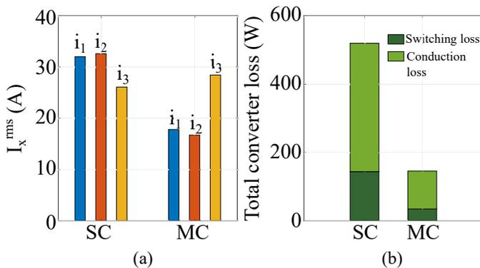
Fig. 8. Comparison of single-current (SC) and multi-current (MC) optimization schemes in terms of a) transformer winding rms currents and b) converter conduction and switching loss;  $V_{DC} = 325V, V_{HV} = 420V, V_{LV} = 48V, P_2 = 3.3kW, P_3 = 1kW$ .
