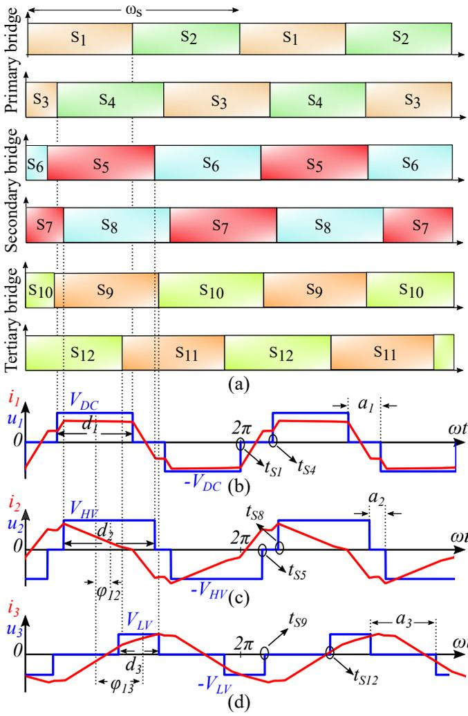
Fig. 5. a) Gate signals of semiconductor devices  $S_1 - S_{12}$  and corresponding voltage and current waveforms of the transformer b) primary, c) secondary and d) tertiary windings.
