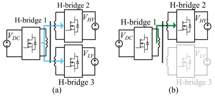
Fig. 4. Charging functions of the proposed integrated charger i.e., a) HV and LV battery simultaneous charging from the grid (G2B), b) individual HV battery charging from the grid (G2H).
