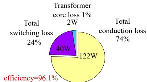
Fig. 15. Power loss breakdown for the converter nominal operating point of  $V_{HV} = 420V$ ,  $P_2 = 3.3kW$ ,  $V_{LV} = 48V$  and  $P_3 = 1kW$  and operation with the total loss optimization scheme
