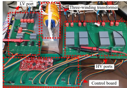
Fig. 11. Experimental setup of TAB converter.
