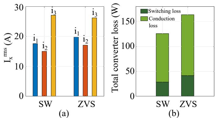
Fig. 9. Comparison of switching loss (SW) and zero-voltages-switching (ZVS) optimization schemes in terms of a) transformer winding rms currents and b) converter conduction and switching loss;  $V_{DC} = 325V, V_{HV} = 395V, V_{LV} = 48V, P_2 = 3.1kW, P_3 = 1kW$ .
