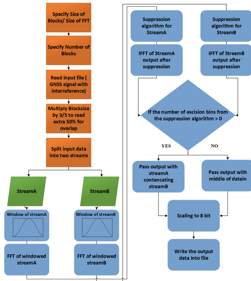
Figure 13. Flowchart of the FFT excision algorithm.
