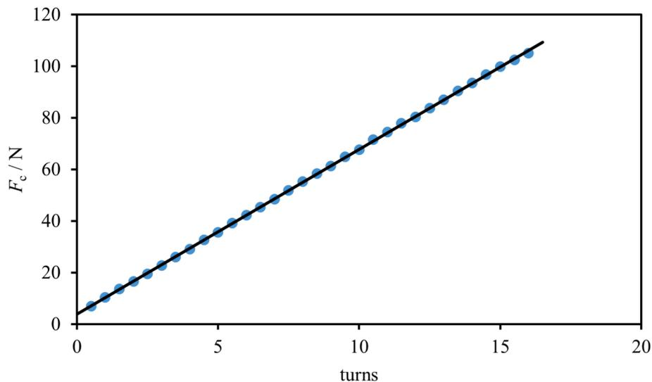
Fig. 2. Compaction force,  $F_c$ , as a function of the number of turns of the jacking screws (for the fixture shown in Fig. 1). The intercept is greater than zero due to the initial tension, which must be overcome in order for the spring coils to start to open. If springs with a different spring constant are used, the calibration curve will be different.
