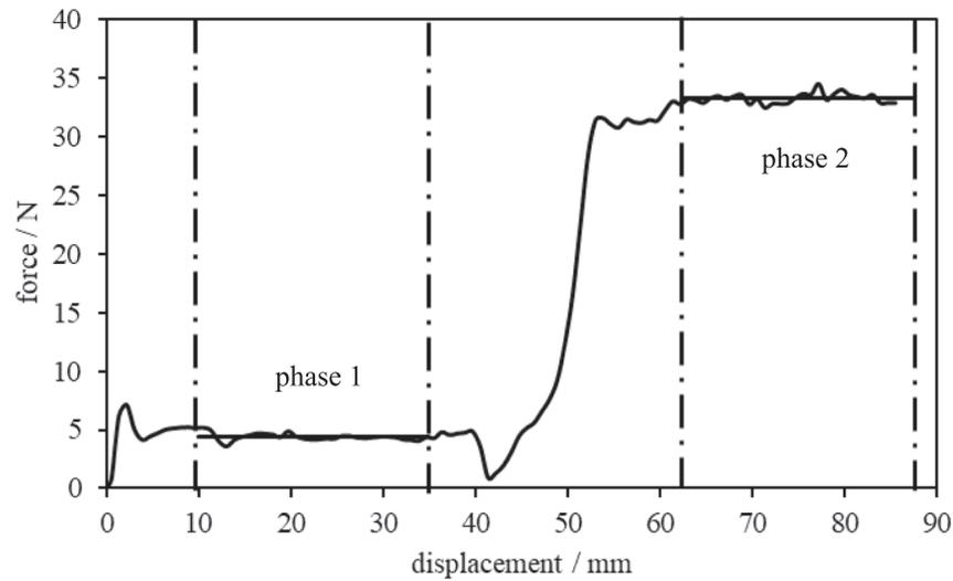
**Fig. 3.** Example of a typical force–displacement data recorded during a tack test on an aerospace-grade prepreg. The peel force as a measure for tack is calculated from the difference between the average values of the indicated force levels during phase 1 and phase 2.
