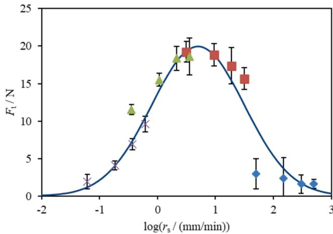
Fig. 5. Example prepreg data from previous work [12] showing the measured tack force,  $F_t$ , as a function of the shifted rate,  $r_s$ , at a reference temperature,  $T_0 = 20$  °C. Error bars indicate standard deviations within each experiment. Different markers indicate data acquired at different test temperatures,  $T$ . A Gaussian fit curve described by Eq. (2) is also shown. Coefficient of determination,  $R^2 = 0.901$ .
