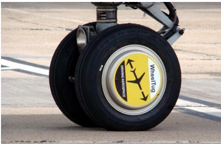
Fig. 6. WheelTug ETS implemented in NLG of B767.
