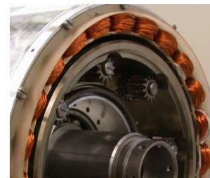
Fig. 7. DLR on-board ETS: view of the rotor with the rim-side double stage planetary gear [64].
