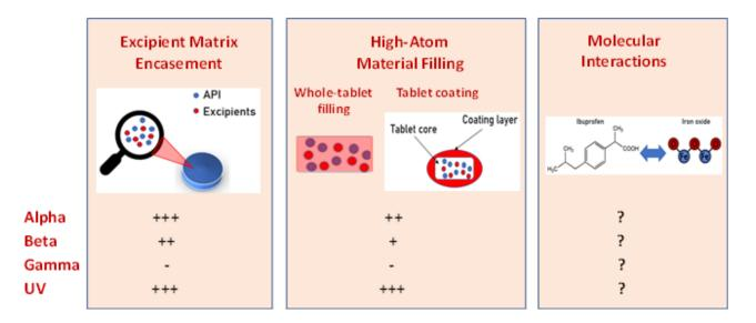
Concepts for radiation shielding used in ISS-MISSE where (+) = expected contribution to radiation protection, and (-) = negligible effect.
