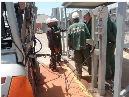
Fig. 7 – Implats representatives demonstrate to seconded HYDRIDE4MOBILITY consortium members (HZG, HYSTORSYS) on-site refuelling of the fuel cell forklift with MH hydrogen storage extension tank. Springs, South Africa, November 2019.
