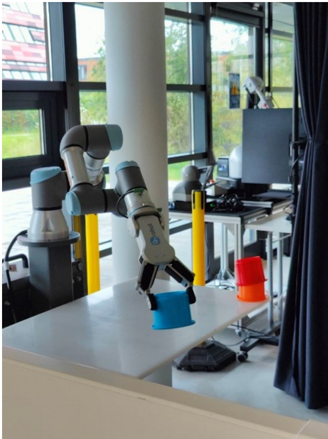
Figure 1: A Universal Robots UR3 robotic arm demonstrating picking up and moving dishes
