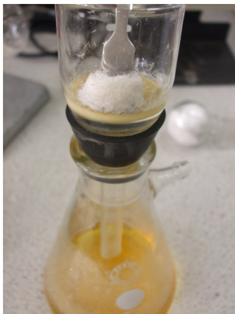
Figure S8: Crude 1 isolated after filtration and aqueous washing. The water soluble photo and acid-catalysts remain in the aqueous solution.
